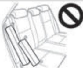
**Note:** The air vent on the right side of the rear seatback is designed to assist in cooling the Hybrid vehicle battery. **DO NOT BLOCK OR COVER THIS VENT**, as it may cause overheating, resulting in reduced vehicle performance.
