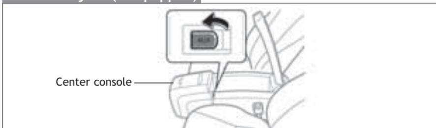
By inserting a mini plug into the AUX audio jack, you can listen to music from a portable audio device through the vehicle's speaker system while in AUX mode.
