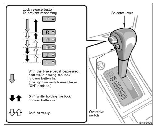
Your automatic transmission has a shift lock system to minimize the possibility of incorrect operation. This means you can only shift out of "P" position when the brake pedal is depressed (with the ignition switch in "ON" position and the lock release button depressed).
