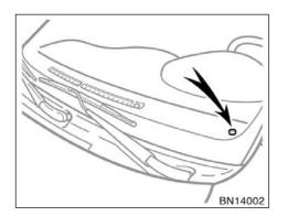
The daytime running light control sensor is on the top of the driver's side instrument panel.
