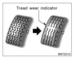
Checking and replacing tires
