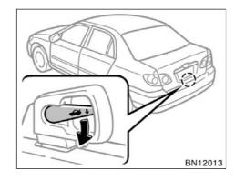
If a person is locked in the trunk, he/she can pull down the phosphorescent handle on the inside of trunk lid to open the trunk lid.
