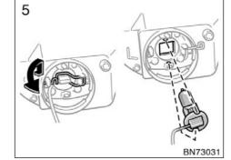
5. Release the bulb retaining spring and remove the bulb. Install a new bulb and the bulb retaining spring.
