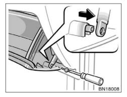
1. Open the glove box. Remove the screw with a Phillips-head screwdriver and slide off the damper as shown.
