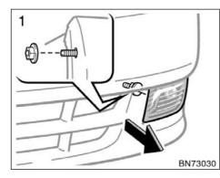
1. Loosen the retainer nut and take out the front fog light unit.
