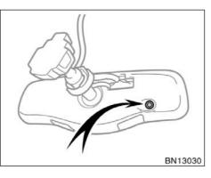
To ensure correct functioning of an anti-glare mirror sensor located on the back side of the mirror, do not touch or cover the sensor with your finger or a piece of cloth, etc.
