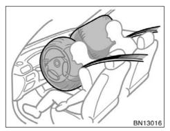
Your vehicle is equipped with a crash sensing and diagnostic module, which will record the use of the seat belt restraint system by the driver when the SRS front airbags are inflated.
