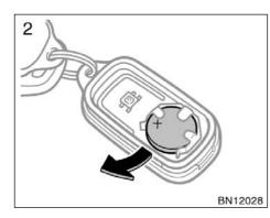
2. Remove the discharged transmitter battery.
