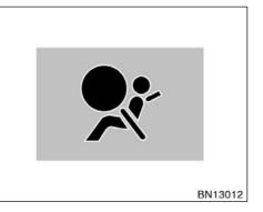
This indicator comes on when the ignition key is turned to the "ON" position. It goes off after about 6 seconds. This means the SRS side airbags are operating properly.
