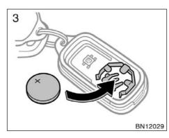
3. Put a new transmitter battery with positive (+) side up.
