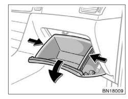
2. Push each side of the glove box to disconnect the claws.
