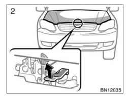
2. In front of the vehicle, pull up the auxiliary catch lever and lift the hood.
