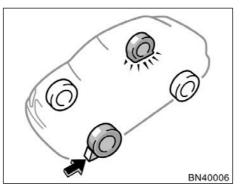
2. Block the wheel diagonally opposite the flat tire to keep the vehicle from rolling when it is jacked up.
