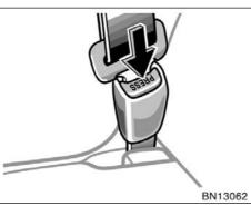
2. To remove the child restraint system, press the buckle release button and allow the belt to retract.
