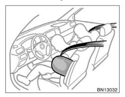
The SRS (Supplemental Restraint System) side airbags are designed to provide further protection for the driver and front passenger in addition to the primary safety protection provided by the seat belts.
