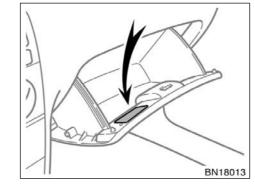
The air conditioning filter information label is placed inside of the glove box as shown and indicates that a filter has been installed.
