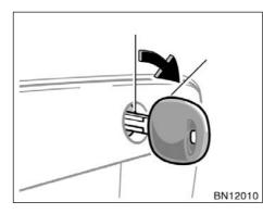
To open the trunk lid from the outside, insert the master key and turn it clockwise.
