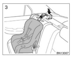
3. Securely fasten the child restraint system with the seat belt.
