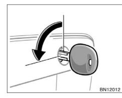
After closing the trunk lid, insert the master key and turn it counterclockwise to deactivate the lock release lever.
