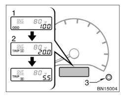
This meter displays the odometer and two trip meters when the ignition switch is on.
