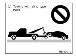
(c) Towing with sling type truck
