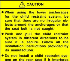
• Do not install a child restraint system on the rear seat if it interferes with the lock mechanism of the front seats. Otherwise, the child or front seat occupant(s) may be killed or seriously injured in case of sudden braking or a collision.
