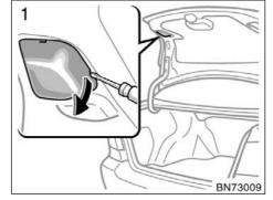
Use a flat-bladed screwdriver or equivalent.
