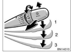
To turn on the windshield wipers, move the lever to the desired setting.
