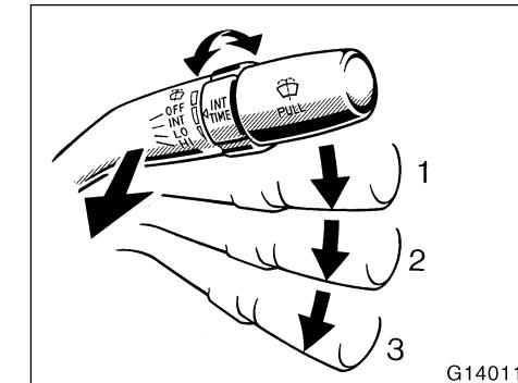
To turn on the windshield wipers, move the lever to the desired setting. The key must be in the "ON" position.
