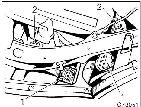
The headlights have the beam angle gauges to check:
