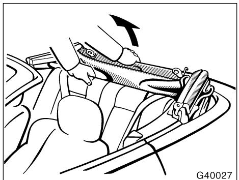
3. From the rear seat, place one hand on top of the rear seatback. With the other hand, grasp the convertible top edge at the center and slowly raise the top half way.
