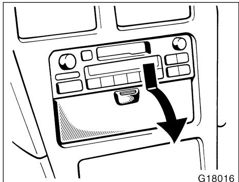
To open the auxiliary box, press on the knob and pull out the box lid.
