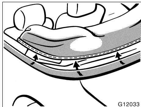
3. Pull out the outer edge of the top boot from under the body moldings.
