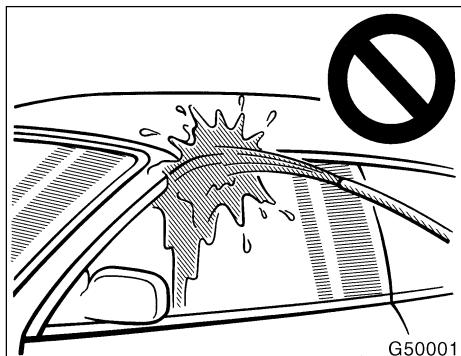
Convertible models: Spray water on the side windows or top seals from above, at a 45° angle to the ground.
