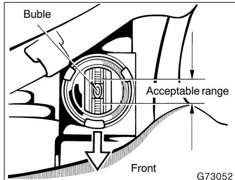
Vertical movement gauges: The bubble on the gauge should be within two marks from center on both sides.
