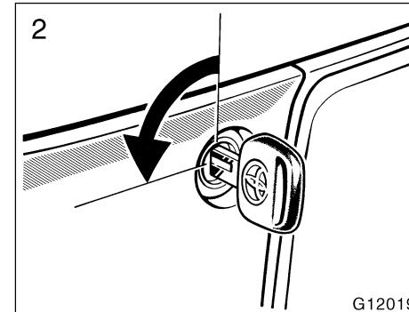
2. After closing the trunk lid or back door, insert the master key and turn it counterclockwise to deactivate the lock release lever.
