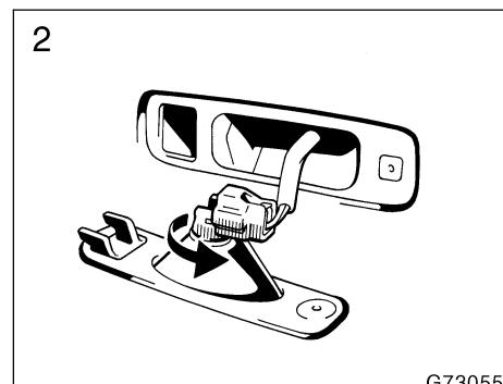
—Rear side marker, rear turn signal, stop and tail, and back-up lights (convertible)
