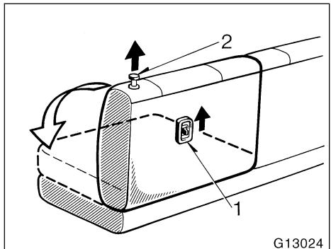
1. Pull up the seatback security lock lever 1 to the unlock position.
