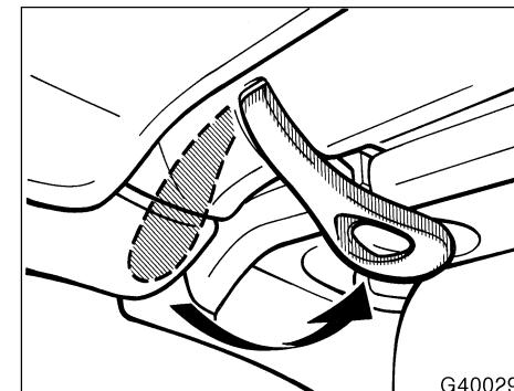
5. While holding the convertible top against the windshield frame, push the latch handles fully forward till they are hooked.
