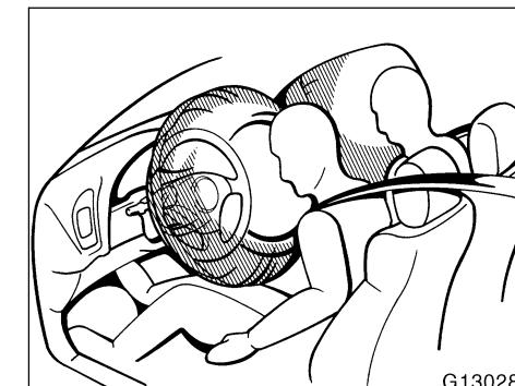
The SRS (Supplemental Restraint System) airbags are designed to provide further protection for the driver and front passenger when added to the primary protection provided by the seat belts.
