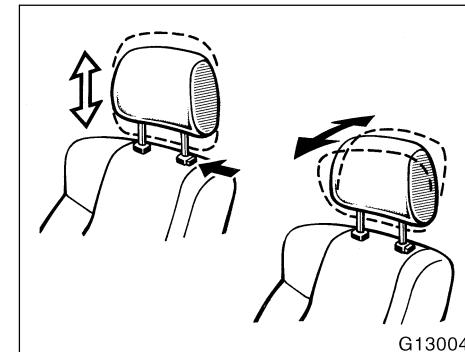
For your safety and comfort, adjust the head restraint before driving.
