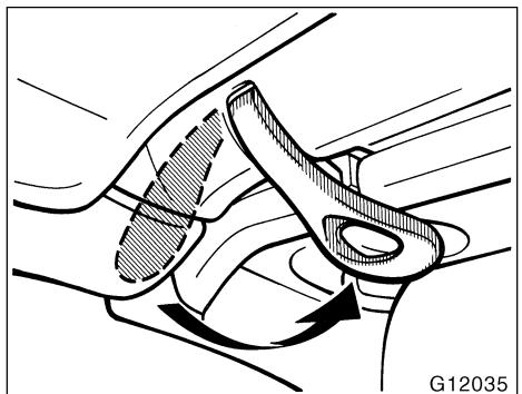
5. Push the latch handles fully forward till they are hooked.
