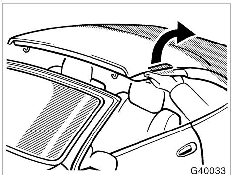
3. Place your palms under either front convertible top side rail around its center and lower the convertible top all the way down. Raise the sun visors.
