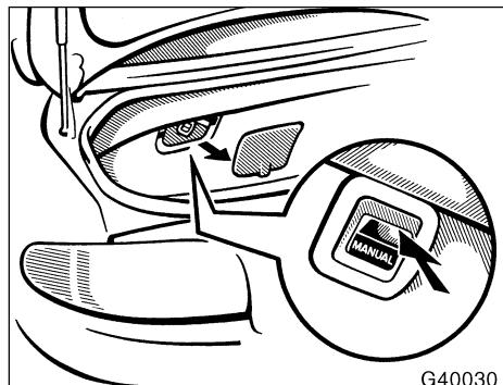
4. Return the manual control switch to the opposite side of the "MANUAL" position, attach the cover, and close the trunk.
