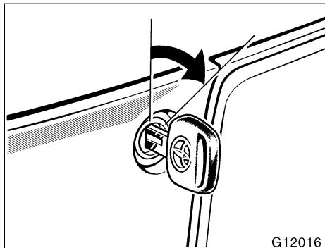
To open the trunk lid or back door from the outside, insert the master key and turn it clockwise.
