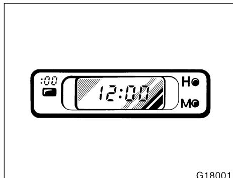
If the electrical power source has been disconnected from the clock, the time display will automatically be set to 1:00 (one o'clock).
