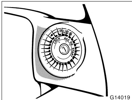
For easy access to the ignition switch, the ignition switch light comes on when either side door or the back door is opened.
