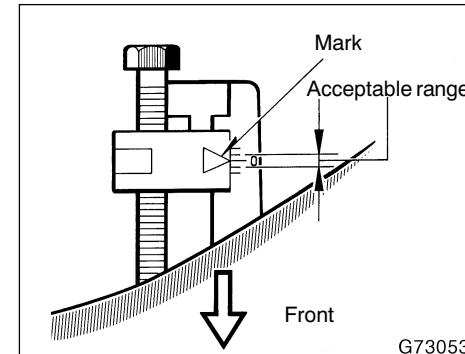
Horizontal movement gauges: The triangle mark on the gauge should be within one mark from the "O" position.
