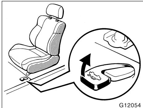
To open the trunk lid or back door from the driver's seat, pull up on the lock release lever.
