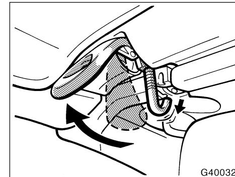
6. Return the manual control switch to the opposite side of the "MANUAL" position, attach the cover, and close the trunk. Raise all the side windows, quarter windows, and sun visors.
