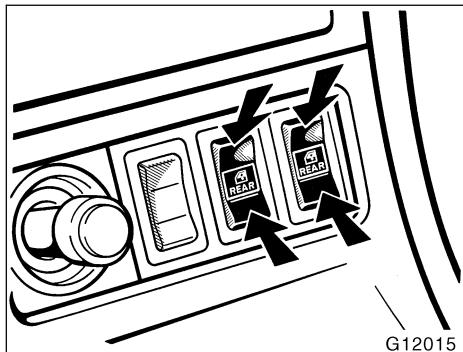
The windows can be operated with switches on the center console.
