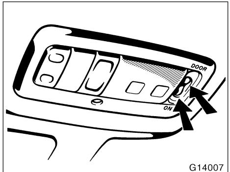
To turn on the interior light, push the switch. To turn the light off, slightly push the switch on the opposite side.
