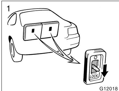
This system deactivates the lock release lever so that things locked in the trunk or luggage compartment can be protected.
