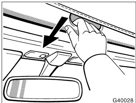
4. Move to the front seat, grasp the handle which is under the convertible top and pull the top fully forward.
