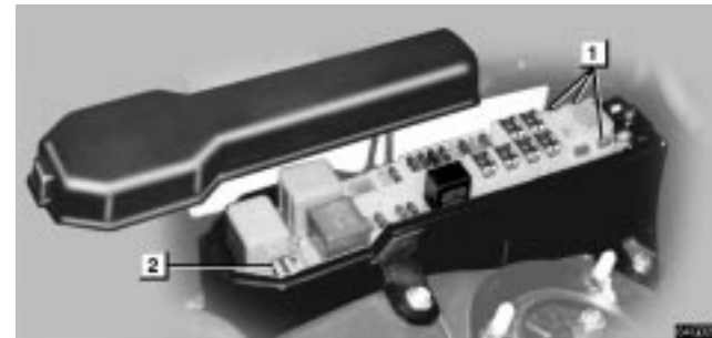
► Engine compartment 1 Spare fuses 2 Pull-out tool
