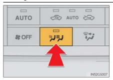
Press the S-FLOW mode button to operate the system.
