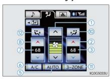
Operations such as changing the air outlets or fan speed are carried out on the screen.
