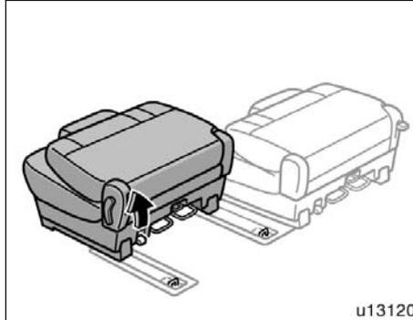
If the seat legs are locked in the wrong position, pull up the left side lever under the seat. Then lift and remove the seat.
