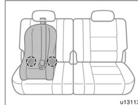
Lower anchorages for the child restraint systems complying with the FMVSS225 or CMVSS210.2 specifications are installed in the right side position of the third seats.
