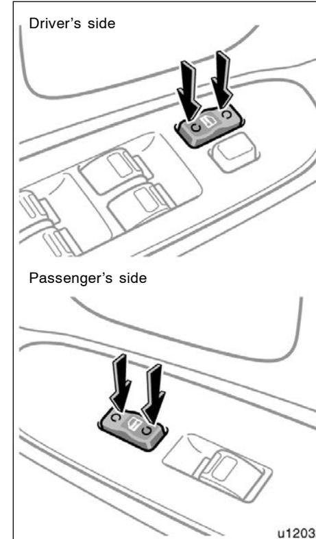
**LOCKING AND UNLOCKING WITH POWER BACK DOOR LOCK SWITCH**
