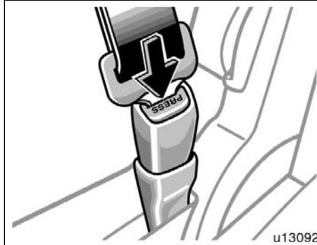
2. To remove the child restraint system, press the buckle release button and allow the belt to retract.
