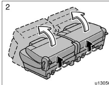
2. Unlock the seat leg by pulling the lock release lever on the rear of the seat cushion and swing the whole seat up and forward.
