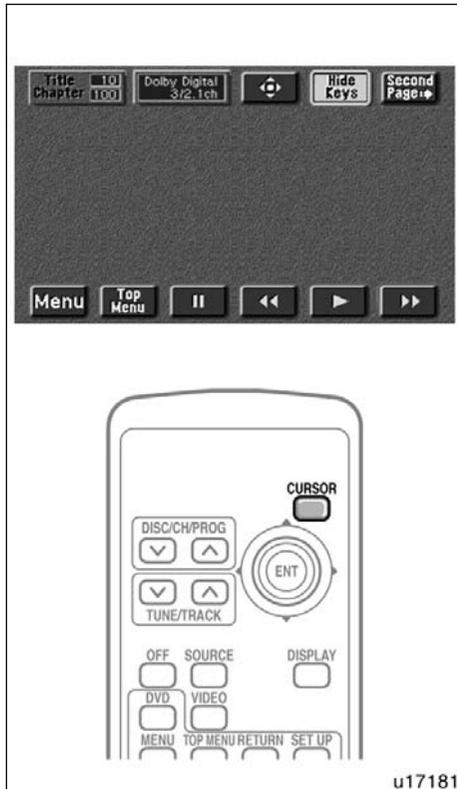
To turn off the switches on the screen, push the “CURSOR” button on the controller once again or push the “Hide Keys” on the screen.
