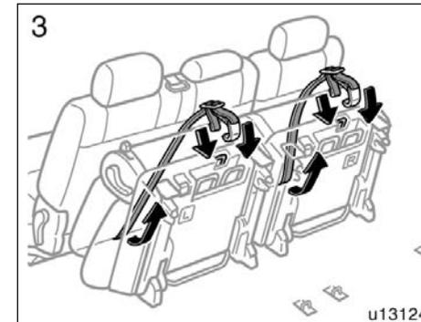
3. Take the holding strap out of its hole which is on the rear of the second seat (For the location of the strap, see “—Tumbling second seats for luggage space” on page 47 in this Section.), and hang the strap onto the anchor. Next, pull the strap on the free end to secure the seat.
