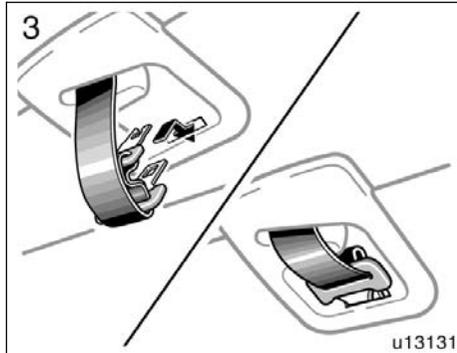
3. To stow the center seat belt, pull it slightly out of its cover. It will automatically roll back partway. Roll the seat belt backwards as shown above and insert it into the slot of its cover. Make sure the tabs are securely locked in the cover.
