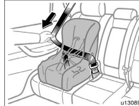
2. Fully extend the shoulder belt to put it in the lock mode. When the belt is then retracted slightly, it cannot be extended.
