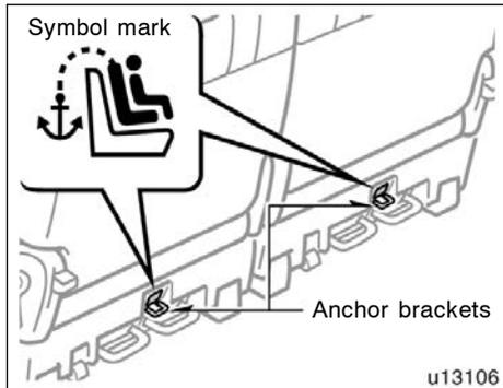
Use the anchorage on the rear of the seatback of each third seat to attach the top strap.
