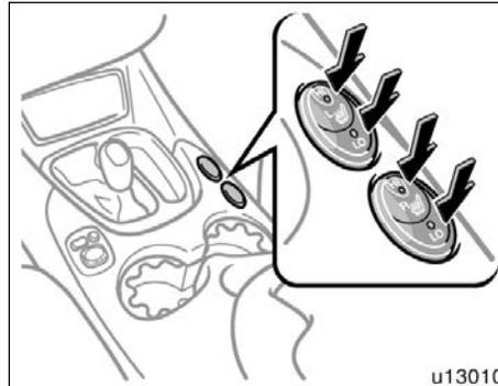
To turn on the seat heater, push the switch to “HI” (high heating temperature) or “LO” (low heating temperature). At this time, the indicator light will illuminate to indicate the seat heater is operating.
