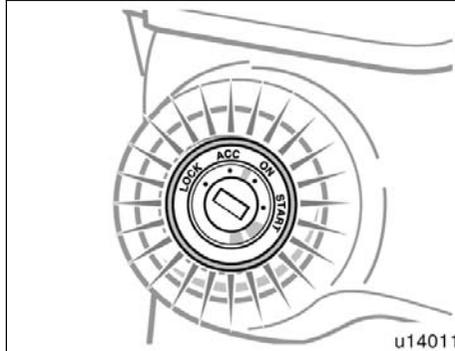
**For easy access to the ignition switch, the ignition switch light comes on when any of the side doors are opened.**
