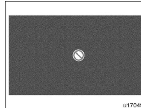
If "⊘" appears on the screen when you select a switch, it indicates that the switch cannot work.
