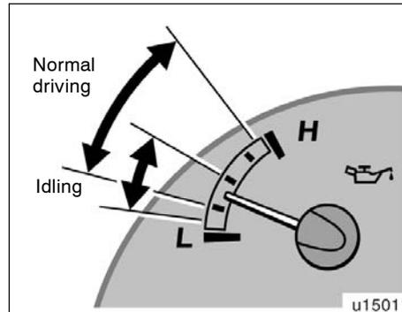
The oil pressure gauge indicates engine oil pressure when the ignition switch is on. Check it while driving to make sure that the needle is in the proper range.
