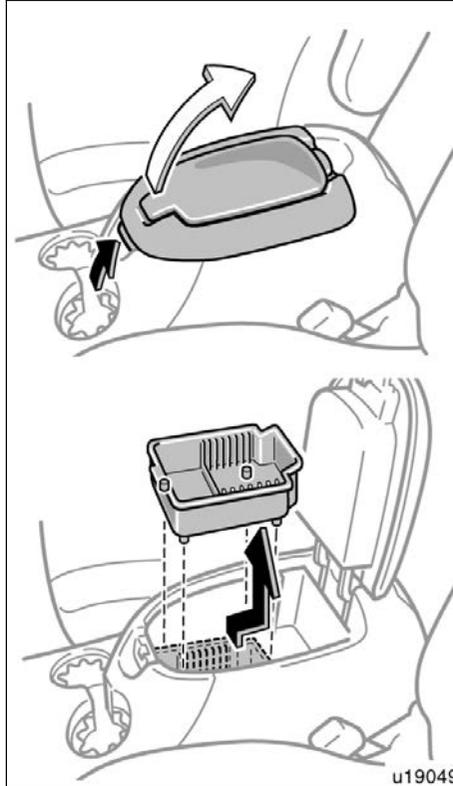
**The rear console box is equipped with compact disc and cassette tape holder.**
