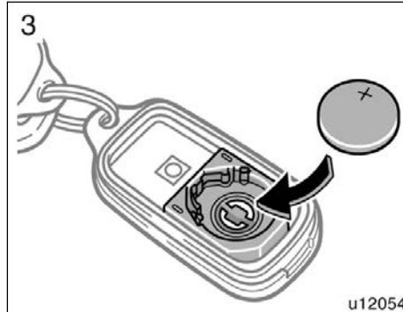
3. Put a new transmitter battery with positive (+) side up.
