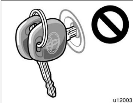
◆ **When starting the engine, do not use the key with other transponder keys around (including keys of other vehicles) and do not press other key plates against the key grip. Otherwise the engine may not start, or may stop soon after it starts. If this happens, remove the key once and then insert it again after removing other transporter keys (including keys of other vehicles) from the ring or while gripping or covering them with your hand to start the engine.**
