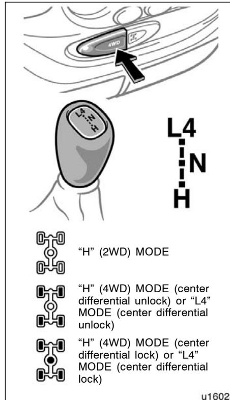
Use the front drive control lever, “4WD” switch and center differential lock switch to select the transfer and center differential modes.
