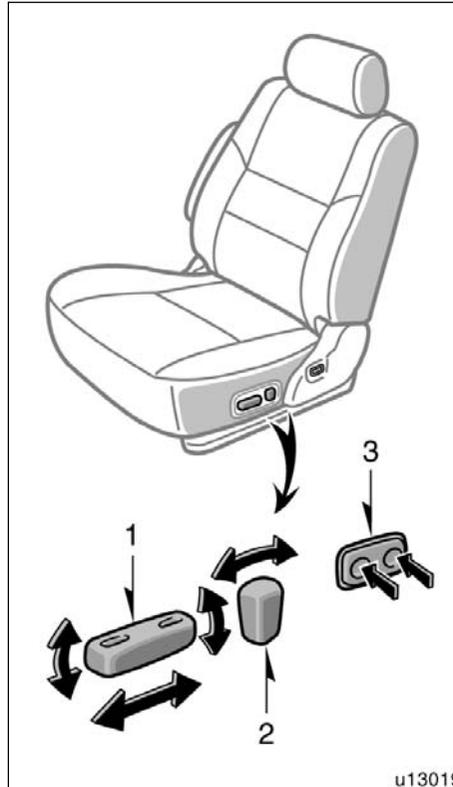
**1. SEAT POSITION AND SEAT CUSHION ANGLE ADJUSTING SWITCH**
