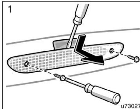
Use a Phillips-head and a flat-bladed screwdrivers. To protect the paint, place several sheets of paper over the paint-work.
