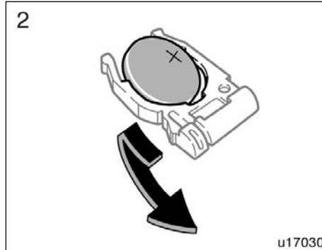
2. Remove the discharged battery.
