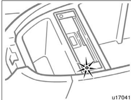
The indicator light turns on while the disc is loaded.
