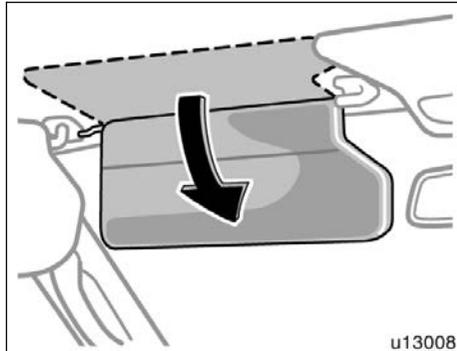
To block the glare from the front when the main sun visor is swung to the lateral side (position 2), swing down the sub visor.
