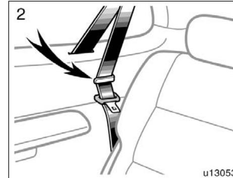
2. When removing the third seats, pass the third seat belts through the hangers.
