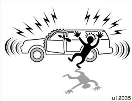
To deter vehicle theft, the system is designed to sound an alarm if any of the side doors, back door or hood is forcibly unlocked or opened or the battery terminal is disconnected and then reconnected when the vehicle is locked. The alarm blows the horn intermittently and flashes the headlights and tail lights.
