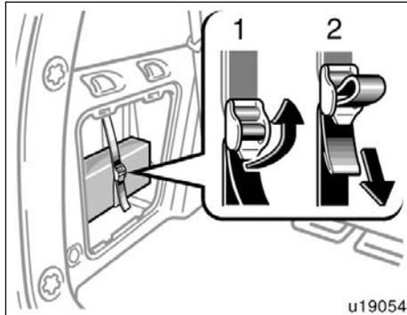
The auxiliary box type E is equipped with a strap to hold the warning reflector.
