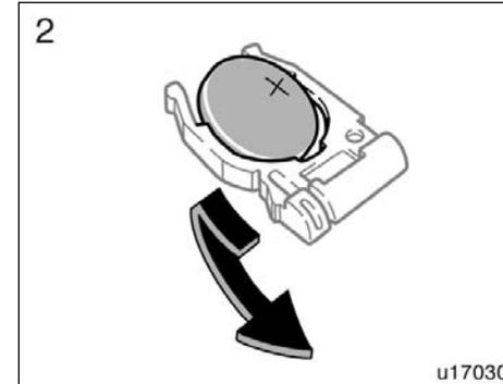
2. Remove the discharged battery.
