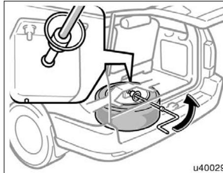
2. Insert the end of the jack handle extension into the lowering screw and turn it counterclockwise with the handle, making sure the handle remains firmly fitted onto the jack handle extension.
