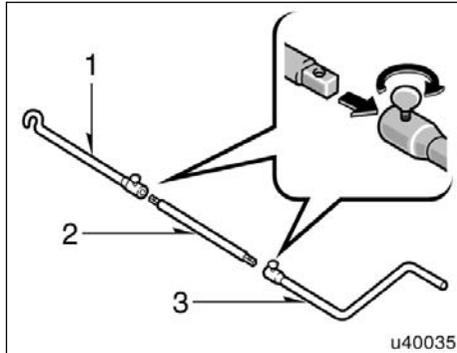
Put a jack handle, jack handle extension and jack handle end together as shown in the illustration.
