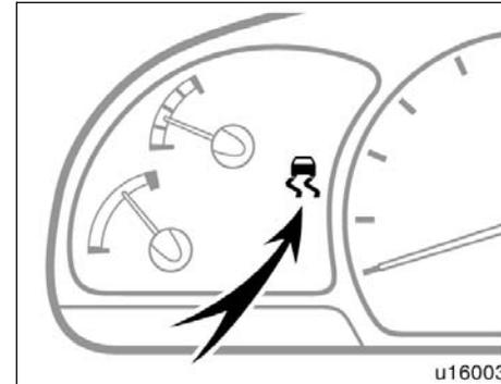
Leave the system on during the ordinary driving so that it can operate when needed.
