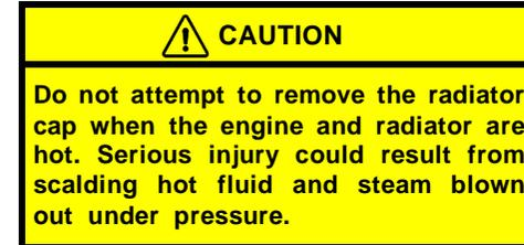
7. After the engine coolant temperature has cooled to normal, again check the coolant level in the reservoir. If necessary, bring it up to half full again. Serious coolant loss indicates a leak in the system. You should have it checked as soon as possible at your Toyota dealer.
