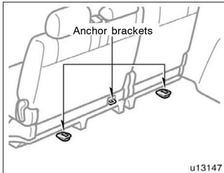
Use one anchorage on the rear of second seats and two anchorages on the floor as shown above to attach the top strap.
