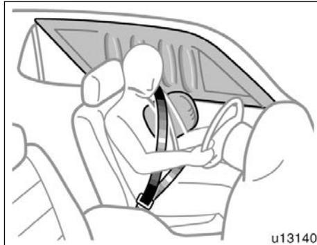
The SRS (Supplemental Restraint System) side airbags and curtain shield airbags are designed to provide further protection for the driver and front passenger in addition to the primary safety protection provided by the seat belts.
