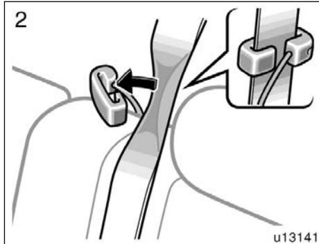
2. Pinch the two edges of the shoulder seat belt for the third seat center position with your fingers and slide the belt past the slot of the guide as shown above. At this time, the elastic cord must be behind the seat belt.
