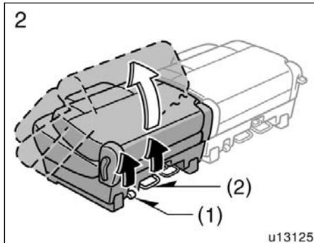
2. Pull the center handle (2) up while holding up the left side lever (1) under the seat, lift the seat and remove it toward you.
