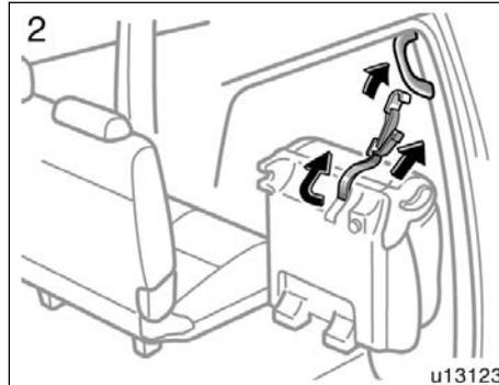
2. Take the holding strap out of its hole, and hook the strap onto the assist grip. Then, pull the strap on the free end to secure the seat.
