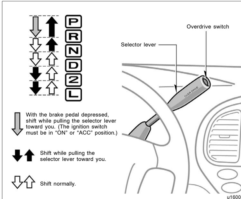
Your automatic transmission has a shift lock system to minimize the possibility of incorrect operation. This means you can only shift out of "P" position when the brake pedal is depressed (with the ignition switch in the "ON" or "ACC" position and the selector lever pulled toward you).
