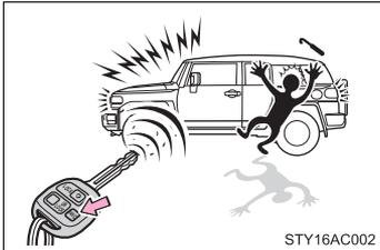
When PANIC button is pushed for longer than about one second, an alarm will sound for about 60 seconds and the vehicle lights will flash to deter any person from trying to break into or damage your vehicle.
