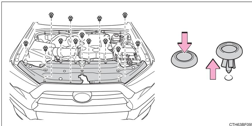
**■ Installing the clips**
