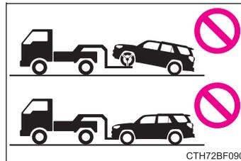
4WD models: Be sure to transport the vehicle with all four wheels raised off the ground. If the vehicle is towed with the tires contacting the ground, the drivetrain or related parts may be damaged, the vehicle may fly off the truck.
