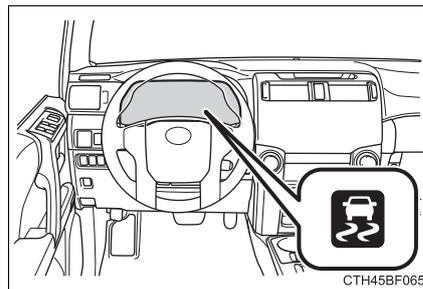
**When the TRAC/VSC/Trailer Sway Control/hill-start assist control systems are operating (4WD models)**
