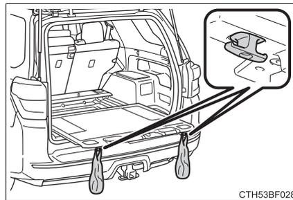
Type B only: To use the grocery bag hooks, slide the slide deck to the full-slide locked position.
