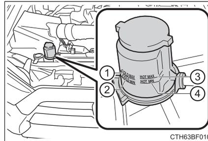
**Hot:** Vehicle has been driven around 50 mph (80 km/h) for 20 minutes, or slightly longer in frigid temperatures. (Fluid temperature, 140°F - 175°F [60°C - 80°C]).
