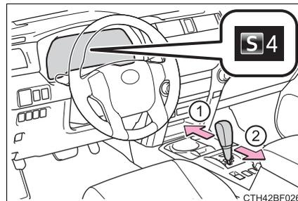
The initial shift range in S mode is set automatically to “4” according to vehicle speed. However, the initial shift range may be set to “3” if AI-SHIFT has operated while the shift lever was in the D position.
