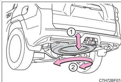
3 Repeat step 2 any time the tire is lowered or disturbed.
