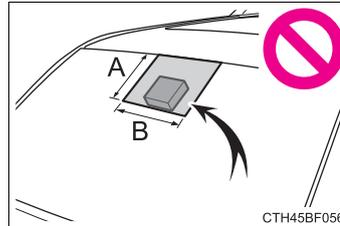
A: From the top of the windshield to approximately 0.4 in. (1 cm) below the bottom of the front camera
