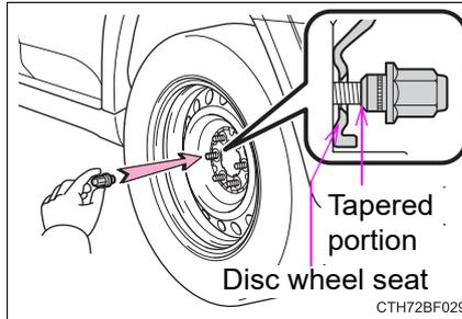
When replacing an aluminum wheel with an aluminum wheel, tighten the wheel nuts until the washers come into contact with the disc wheel.
