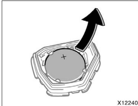
4. Take out the discharged battery and put in a new battery with the positive (+) side up.
