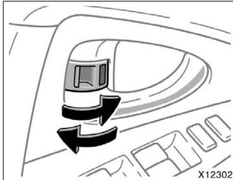
**LOCKING AND UNLOCKING WITH INSIDE LOCK KNOB**
