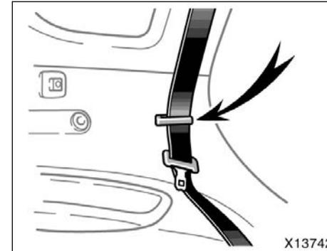
3. Make sure the outer seat belt passes through the hanger when folding the rear/second seat.
