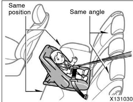
● When installing a child restraint system on the rear/second center position, adjust both seat cushions to the same position and align all seatbacks at the same angle. Otherwise, the child restraint system cannot be securely restrained and this may cause death or serious injuries in a collision.
