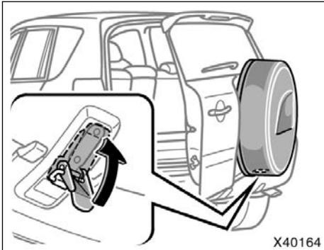
3. Open the back door. Lock the latch handle which is on the bottom of the cover.
