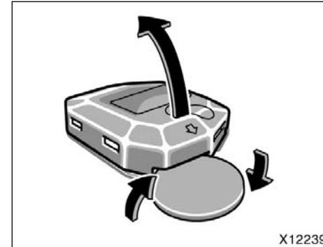
3. Open and remove the battery case cover using a coin.
