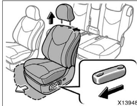
2. Remove the front head restraint. Push the seat position adjusting switch forward to slide the seat to the front-most position.
