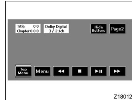
You can select the menu for the disc by the joystick and the “ENT” button on the controller.
