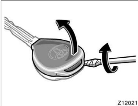
1. Open the cover using a flathead screwdriver wrapped with plastic tape.
