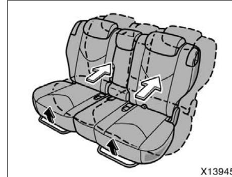
1. Hold the center of the lever and pull it up. Then slide the rear/second seats fully backward and pull it forward slightly until it locks.
