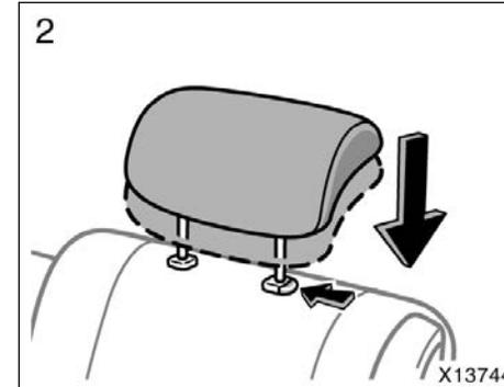
2. Lower the head restraint to the lowest position.
