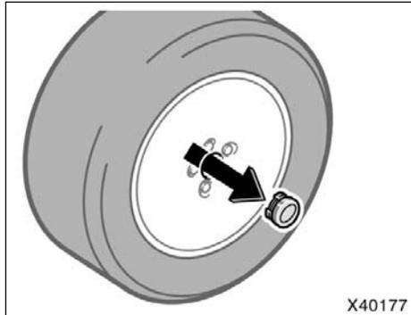
On some models—Before stowing the flat tire, remove the center wheel ornament by pushing from the reverse side.
