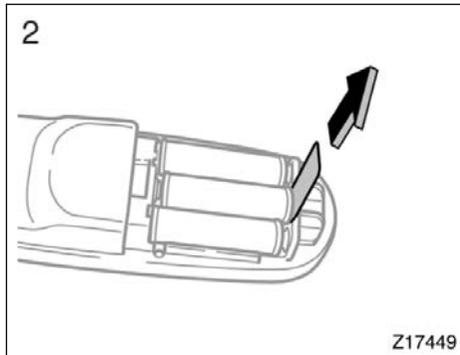
2. Remove the insulating sheet.
