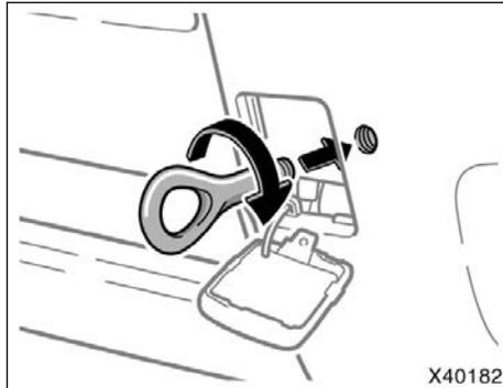
2. Use the front towing eyelet in the tool bag. Secure it to the hole on the bumper by turning clockwise. (For the tool bag location, see “—Required tools and spare tire” on page 356 in this Section.)
