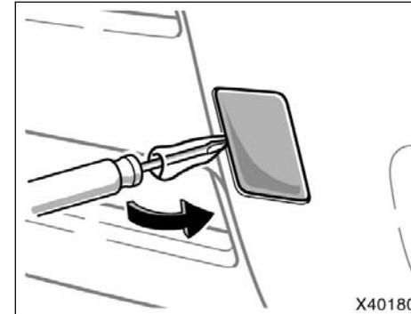
1. Remove the front towing eyelet cover on the front bumper, using a flathead screwdriver which is wrapped with a cloth.
