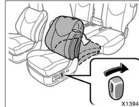
3. Move the seatback angle adjusting switch backward to flatten the seatback.
