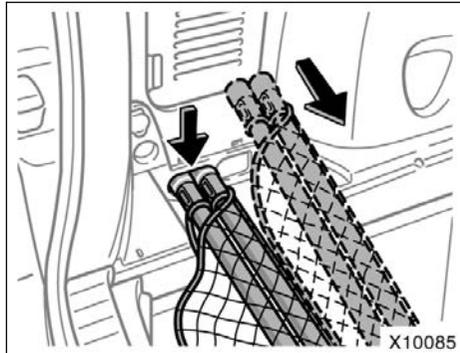
4. Compress the left end of the rear cargo net, and fit it into the other side of the luggage storage box.
