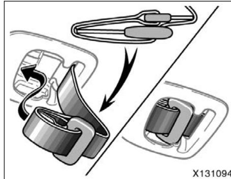
2. Insert the tabs of the center seat belt into the cover. Make sure the tabs are securely locked in the cover.
