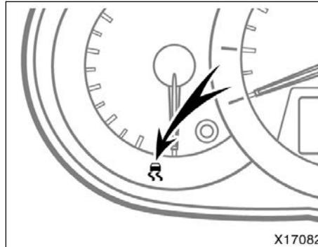
With the vehicle traveling at a speed of 25 km/h (15 mph) or less, release the brake pedal and accelerator pedal to activate the system. The vehicle will descend the hill at a low speed.
