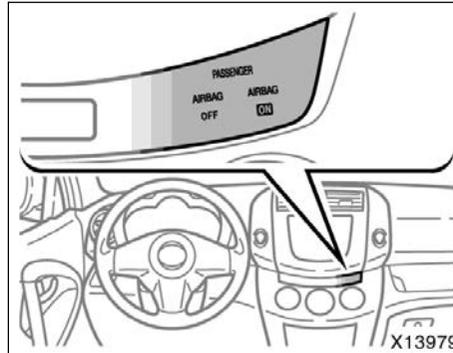
The “AIRBAG ON” and “AIRBAG OFF” indicator lights indicate the actuation of the front passenger airbag, side airbag on the front passenger seat and front passenger’s seat belt pretensioner.
