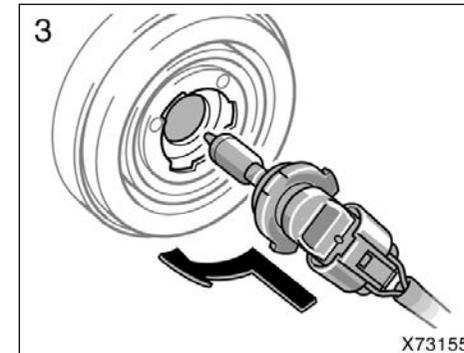
**3. Plug in a new bulb into the connector and install it into the mounting hole.**
