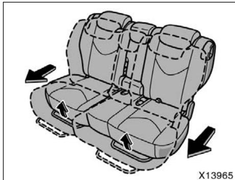
Hold the center of the lever and pull it up. Then slide the rear/second seats forward slightly if it is in the rear-most position.
