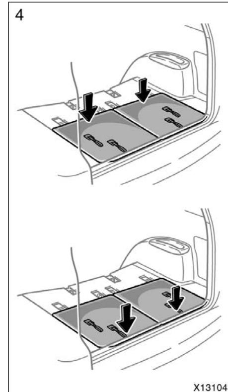
4. Push the seat on the front side against the floor and push the seat on rear side against the floor. Make sure it is locked securely.
