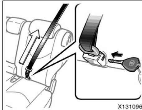
Rear/second center seat: If the seat in which a child restraint system is installed in the rear most position, release the center seat belt after removing the child restraint system. Otherwise, the rear center seat belt may not work properly.
