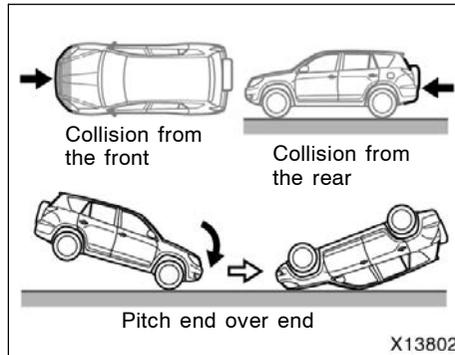
The curtain shield airbags are not generally designed to inflate if the vehicle is involved in a front or rear collision, if it pitches end over end, or if it is involved in a low-speed side collision.
