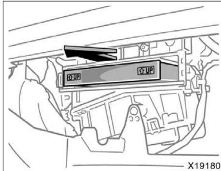
4. Pull the filter out of the filter outlet.
