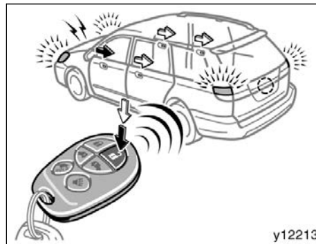
Unlocking operation (type B or C)
