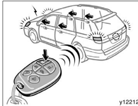
Locking operation (type B or C)
