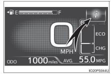
2 Press or of the meter control switches to select the display item.
