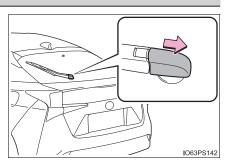
2 Move the wiper blade until a click sound can be heard and the claw detaches, and then remove the wiper blade from the wiper arm.
