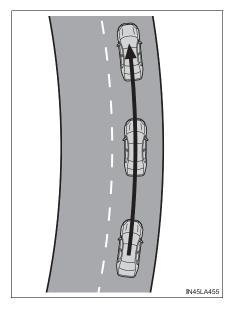
If the system detects that the steering wheel has not been operated for a fixed amount of time or the steering wheel is not being firmly gripped, a warning is displayed on the multi-information display and the function is temporarily canceled.
