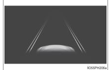
Indicates that the system is recognizing white (yellow) lines or a course\*. When the vehicle departs from its lane, the white line displayed on the side the vehicle departs from flashes orange.
