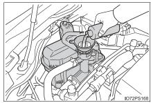
6 Start the hybrid system and turn the air conditioning system on to check that the radiator cooling fans operate and to check for coolant leaks from the radiator or hoses.
