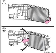
5 Remove the dust and clogs from the filter using a vacuum cleaner, etc.
