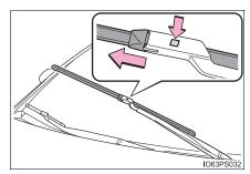
2 Align the wiper blade with the connecting portion of the wiper arm, and then slide it in the direction it was removed from
