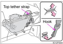
If the head restraint does not interfere with the child restraint system installation, install the head restraint.
