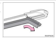
When installing a new wiper insert, perform the procedure in reverse.
