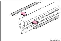
Insert the wiper insert starting from the claw at the center of the wiper blade. Pass the wiper insert through the 3 claws so that it sticks out from the stopper, and then pass the wiper insert through the final remaining claw.
