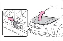
3 Hold the hood open by inserting the supporting rod into the slot.
