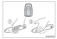
Make sure to touch the sensor on the back of the handle.
