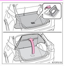
2 Secure the deck board using the grocery bag hooks. (→P. 469)
