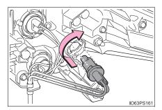
7 Align the grooves on the light unit with the claws, and insert the light unit straight so that the 2 pins on the light unit fit into the holes. Confirm that the light unit is completely secured.
