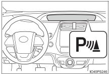
Once off is selected, the intuitive parking assist will not return to on until it is turned to on by the system does not automatically return to on even when the hybrid system is restarted.)
