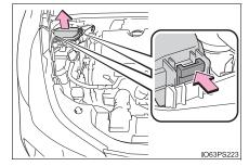
▶ Engine compartment type B fuse box
