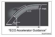
It is easier to drive in an Eco-friendly manner by driving according to the display showing the accelerator pedal operations and staying within the "ECO Accelerator Guidance" range. (→P. 229)
