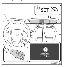
1 Press the "ON-OFF" button to activate the cruise control.
