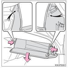
4 With the glove box fully open, slightly lift up the glove box and pull toward the seat to detach the bottom of the glove box.
