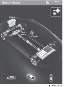
When the vehicle is powered by the gasoline engine
