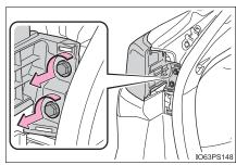
3 Pull the light unit toward the rear of the vehicle to remove it.
