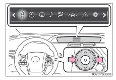
Screens linked with vehicle functions may be automatically displayed according to the operation status of the corresponding functions.
