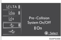
3 When the setting screen is displayed, select the setting or desired value (time, etc.) with the meter control switches.\*1, 2
