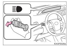
2 Press the Automatic High Beam switch.
