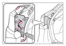
To prevent damage to the cover, protect the tip of the screwdriver with a rag.
