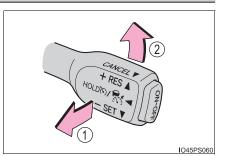
② Pushing the lever up resumes the cruise control and returns vehicle speed to the set speed.
