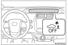
When the Parking Support Brake function is switched off, system operation does not resume until the function is switched back on through the screen on the multi-information display. (System operation does not resume by operating the power switch.)
