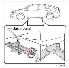
5 Assemble the jack handle and the wheel nut wrench as shown in the illustration.
