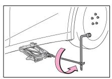
4 Securely tighten the wheel nuts two or three times in the order shown in the illustration using a wheel nut wrench.
