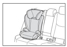
4 Sit the child in the child restraint system. Fit the seat belt to the child restraint system according to the manufacturer's instructions and insert the plate into the
