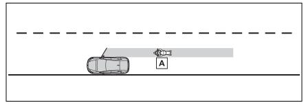
A Vehicle or bicycle which has a high possibility of colliding with a door (other than the back door) when opened
