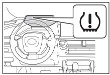
9 If the specified tire inflation pressure of the wheel set installed differs from that of the previous set, it will be necessary to perform the tire inflation pressure setting procedure of the tire pressure warning system. (→P.520)
