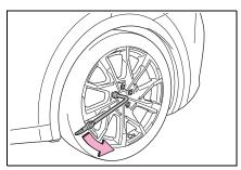
4 Turn the tire jack portion A by hand until the notch of the jack is in contact with the jack point.
