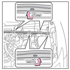
2 Disconnect the claws and remove the service cover.
