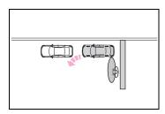
When the vehicle has been parked on a curb and a side sensor detects the road surface 5
