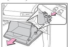
5 Unlock the filter cover (A), pull the filter cover out of the
