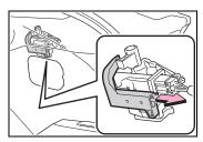
After operating the connector lock emergency release lever, push it back to its original position until a click sound is heard.
