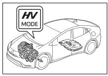
When in HV mode, the vehicle is driven using both the gasoline
