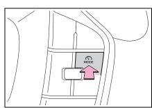
2 Using the accelerator pedal, accelerate to the desired vehicle speed (approximately 20 mph [30 km/h] or more), and press the driving assist switch to set the set vehicle speed.
