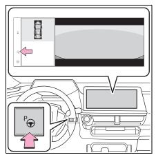
3 Select perpendicular parking (forward/reverse) function or parallel parking function.
