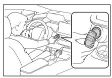
3 Firmly depress the brake pedal and check that and a message are displayed
