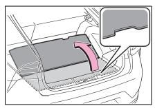
Hold the handle and pull it toward you, and then the 3 clips will be disengaged
