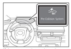
If the system determines that the accelerator pedal is strongly depressed, the following icon and message will be displayed on the multi-information display.
