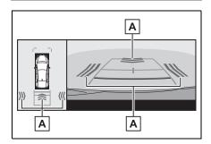
A Pedestrian detection icon Displayed automatically when a pedestrian is detected behind the vehicle.
