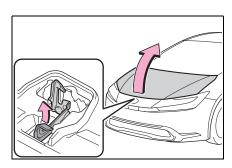
3 Hold the hood open by inserting the supporting rod into the slot.
