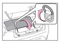
**3** When using the front cargo hook, raise the hook without opening the deck board.
