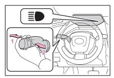
With the headlights on, push the lever away from you to turn on the high beams. 5
