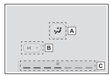
A Select the air flow mode Each time the switch is touched, the air flow mode changes.
