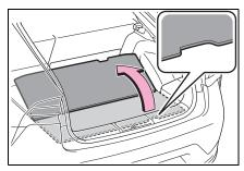
2 Hold the handle and pull it toward you, and then the 3 clips will be disengaged
