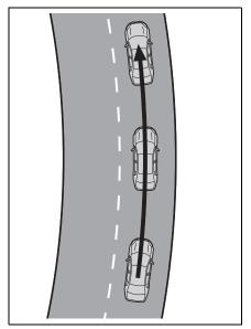
When the function is operating, if the vehicle is likely to depart from its lane, the driver will be alerted via a display and buzzer.
