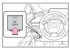
3 Open the lid, and fully and securely insert the plug of the device into the power outlet. (→P.474)
