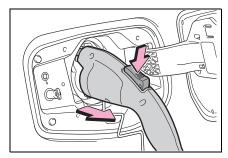
3 Attach the charging connector cap.
