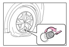
6 Extend the hose. Remove the air release cap from the hose.
