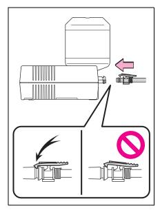
5 Remove the valve cap from the valve of the punctured tire.
