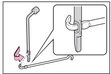
6 Raise the vehicle until the tire is slightly raised off the ground.
