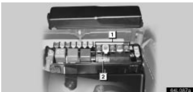
► Engine compartment 1 Spare fuses 2 Pull-out tool
