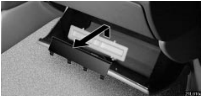
1. Open the glove box and remove the two covers.
