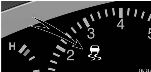
✕ Slip indicator light
