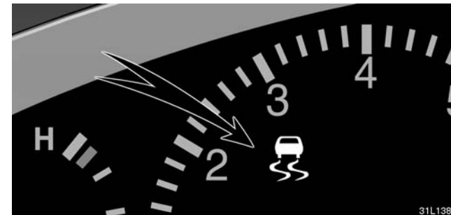
► Slip indicator light
