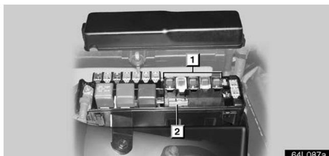
► Engine compartment 1 Spare fuses 2 Pull-out tool
