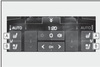
**A** Adjust the rear seat heater temperature level
