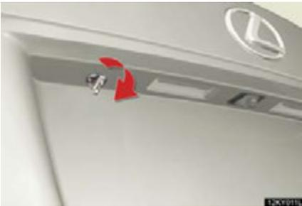
Turn the mechanical key clockwise to open.
