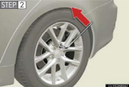
Slightly loosen the wheel nuts (one turn).
