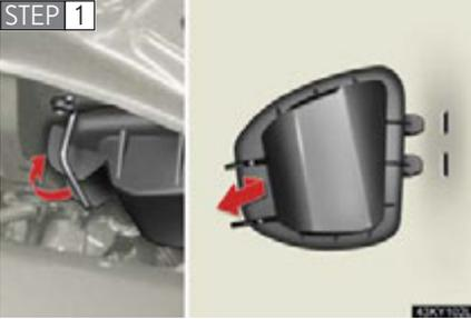
Release the lock and remove the cover.
