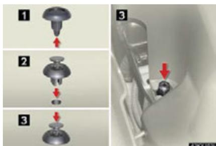
**1** Press the tip of the clip against a hard surface, such as a desk, to allow the center part of the clip to be pushed up.
