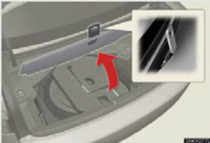
The lever can be hooked on the edge of the trunk.
