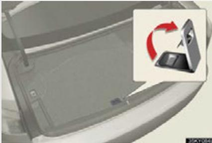
Pull the lever upwards when lifting the luggage mat up.
