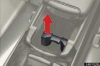
Remove the cup holder insert by holding the base part.
