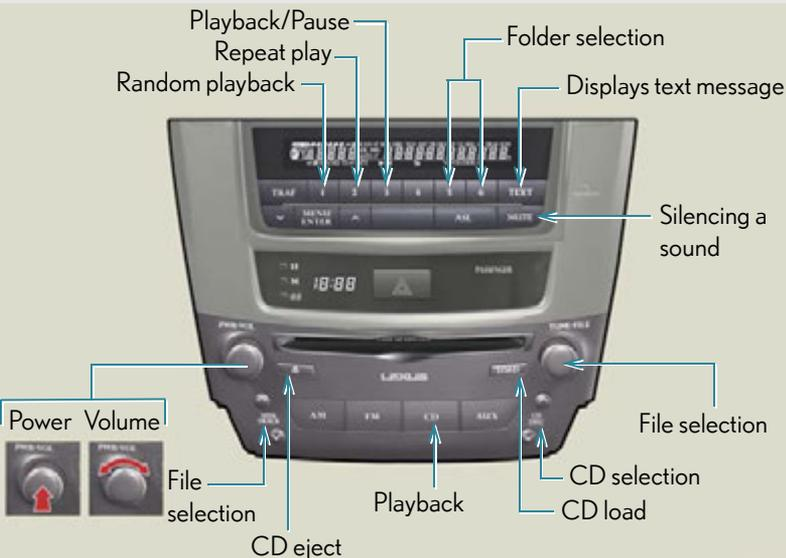
**Loading and ejecting MP3 and WMA discs**
