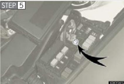
Remove the fuse with the pull-out tool.
