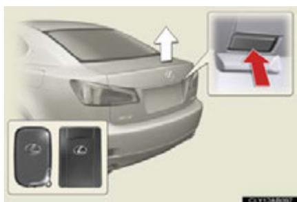
Press the button to unlock the trunk.
