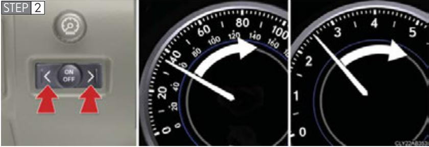
Push “<” or “>” within 6 seconds of the speedometer or tachometer needle moving to change the setting of the desired speed, then turn the indicator mode to “ON” by pushing the “ON/OFF” button.
