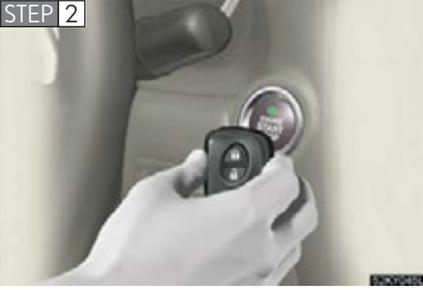
Touch the Lexus emblem side of the electronic key to the “ENGINE START STOP” switch.
