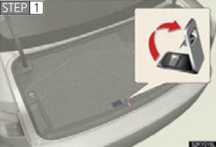
Lift up the hook of the panel on the trunk floor.
