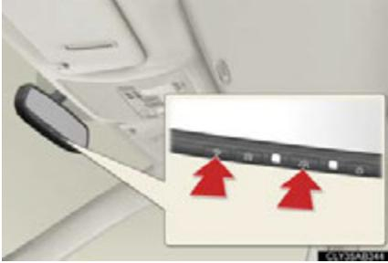
Press and hold the 2 outside buttons for 10 seconds until the indicator light flashes.
