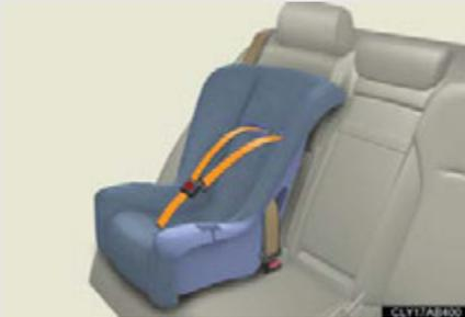
Seat belts equipped with a child restraint locking mechanism (ALR/ELR belts except driver's seat belt) (→P. 66)
