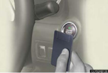
**STEP 3** Press the “ENGINE START STOP” switch within 10 seconds after the buzzer sounds, keeping the brake pedal depressed.
