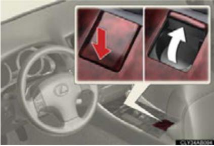
To open, press down and release the front of the cup holder lid.
