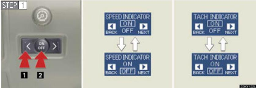
Push “<” or “>” to select the speed or tacho indicator set mode. (1) Turn the speed or tacho indicator to “OFF” and then “ON” by pushing the “ON/OFF” button. (2)
