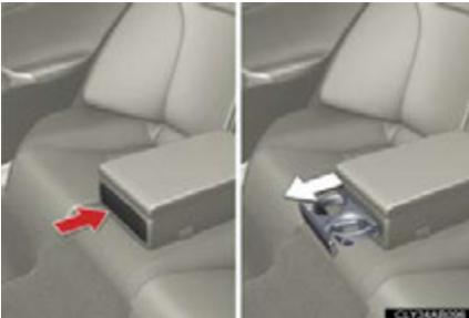
To open, press in and release the rear cup holder on the rear center armrest.
