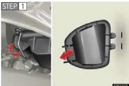
Release the lock and remove the cover.
