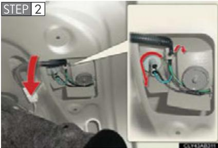
Partly remove the trunk panel cover and turn the bulb base counterclockwise.
