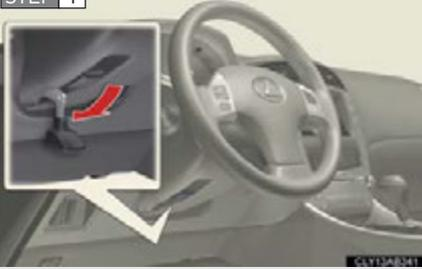
Hold the steering wheel and press the lever down.
