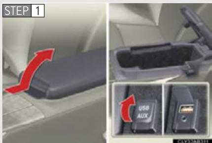
Open the cover and connect the portable audio device.
