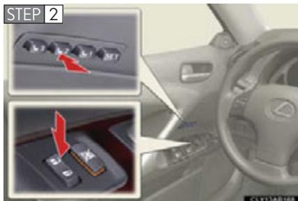
While pressing the desired button (“1”, “2” or “3”), press the lock or unlock side on the driver's door lock switch until the signal beeps.
