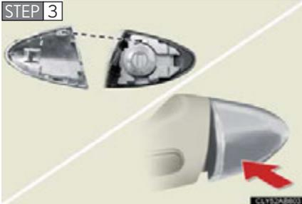
After the operation is completed, reinstall the cover.
