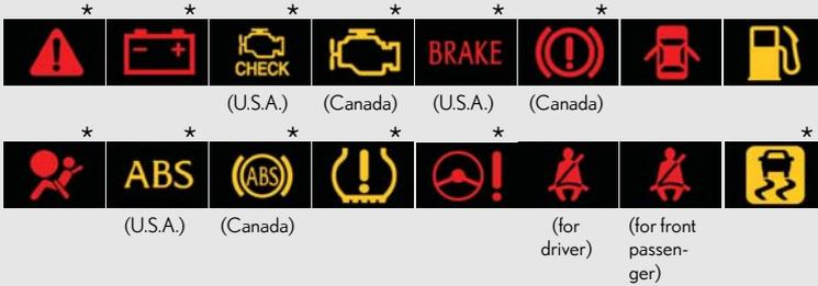
\*: These lights turn on when the “ENGINE START STOP” switch is turned to IGNITION ON mode to indicate that a system check is being performed. They will turn off after the engine is started, or after a few seconds. There may be a malfunction in a system if a light does not come on, or if the lights do not turn off. Have the vehicle inspected by your Lexus dealer.
