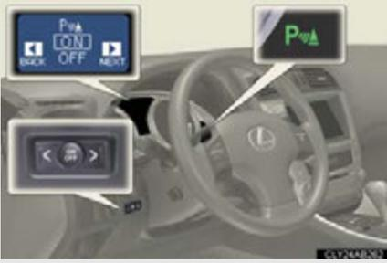
When on, an indicator is displayed to inform the driver that the function is operational.
