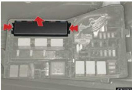
Lift the lid off while pushing the tabs on either side.
