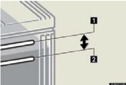
Check that the level is between “UPPER LEVEL” and “LOWER LEVEL”.
