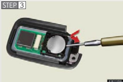
Remove the depleted battery.
