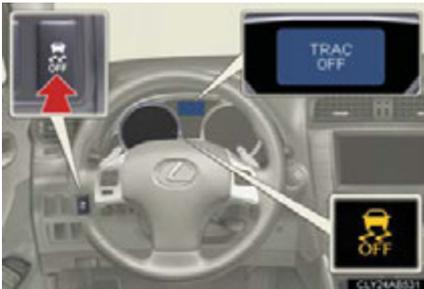
Push and hold the switch for more than 3 seconds or more while the vehicle is stopped to turn off TRAC and VSC.
