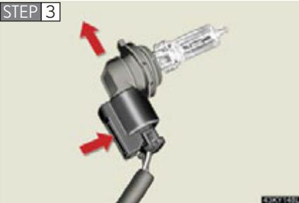
Unplug the connector while depressing the lock release.
