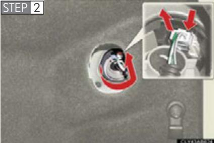
Remove the connector and turn the bulb base counterclockwise.
