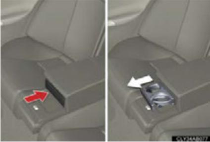
Press in and release the cup holders on the rear center armrest.
