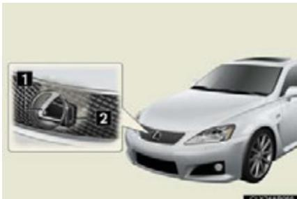
Detects vehicles or other obstacles on or near the road ahead and determines whether a collision is imminent based on the position, speed, and heading of the obstacles.
