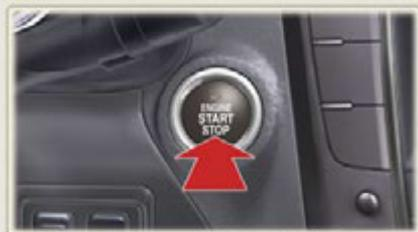
Press the “ENGINE START STOP” switch.
