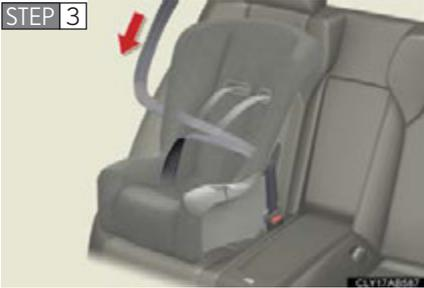
Fully extend the shoulder belt and allow it to retract to put it in lock mode.
