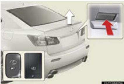
Press the button to unlock the trunk.
