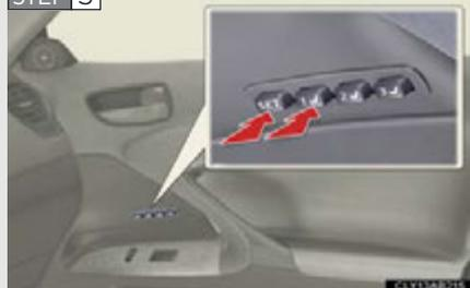
Push the "SET" button, then within 3 seconds push button "1", "2" or "3" until the signal beeps.
