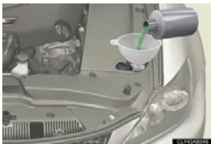
If any washer does not work or the warning message appears on the multi-information display, the washer tank may be empty. Add washer fluid.
