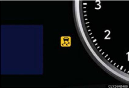
The slip indicator light flashes to indicate that the VSC/TRAC/hill-start assist control systems have been engaged.
