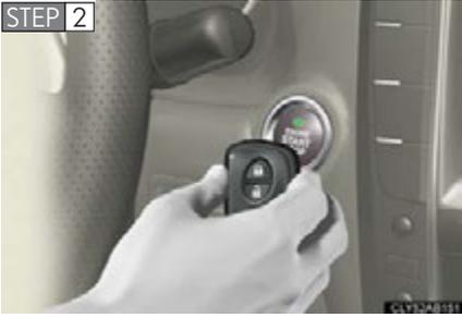
Touch the Lexus emblem side of the electronic key to the “ENGINE START STOP” switch.
