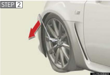
Slightly loosen the wheel nuts (one turn).
