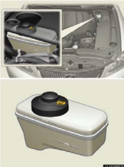
The brake fluid level should be between the “MAX” and “MIN” lines on the tank.
