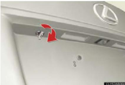
Turn the mechanical key clockwise to open.
