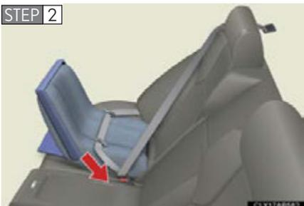
Run the seat belt through the child seat and insert the plate into the buckle. Make sure that the belt is not twisted.
