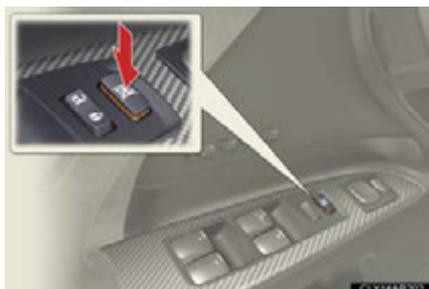
Press the switch down to lock the passenger window switches.
