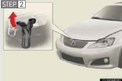
Lift the auxiliary catch lever and lift the hood.
