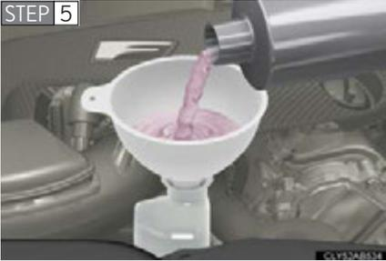
Add engine coolant if necessary.
