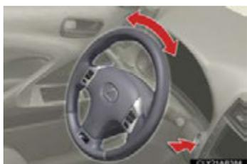
The “ENGINE START STOP” switch indicator will flash in green and a message will be shown on the multi-information display. Press the “ENGINE START STOP” switch again while turning the steering wheel left and right.
