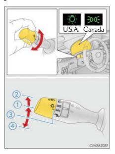
1 With the headlights on, push the lever away from you to turn on the high beams.
