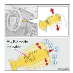
With AUTO mode selected, the wipers will operate automatically when the sensor detects falling rain. The system automatically adjusts wiper timing in accordance with rain volume and vehicle speed.
