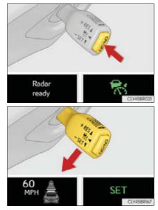
To change the set speed, operate the lever until the desired set speed is displayed.
