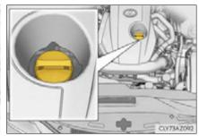
Make sure to check the oil type and prepare the items needed before adding oil.
