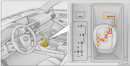
While the engine switch is in IGNITION ON mode, move the shift lever with the brake pedal depressed.
