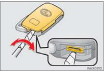
Remove the depleted battery.
