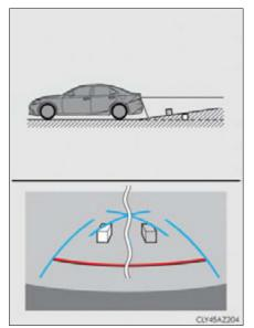
• When the ground behind the vehicle slopes down sharply
