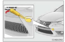
Insert the towing eyelet into the hole and tighten partially by hand.
