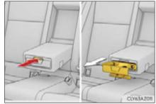
To open, pull down the armrest and press the button and release the rear cup holder on the armrest.
