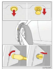
2 Unfasten the clamp, and pull back the fender liner.
