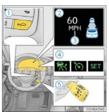
Note that vehicle-to-vehicle distance will close in when traveling on long downhill slopes.
