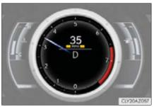
The indicator will illuminate in yellow at an optionally set speed and red at the fixed high speed.
