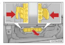
Femove the air conditioning filter from the filter case and replace it with a new one.
