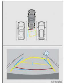
Once the vehicle width guide lines and the parking space lines are parallel, straighten the steering wheel and back up slowly until the vehicle has completely entered the parking space.
