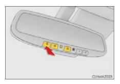
If the indicator light blinks rapidly for 2 seconds and then turns into a solid/continuous light, proceed with the following instructions 4 for programming a rolling code system.
