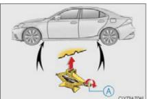
4 Raise the vehicle until the tire is slightly raised off the ground.
