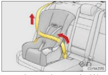
If the child restraint has a top tether strap, the top tether strap should be latched onto the top tether strap anchor.  $(\rightarrow P. 65)$
