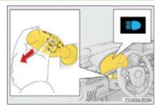
**2** Press the Automatic High Beam switch.
