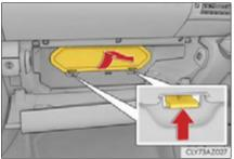
4 Press the tabs and remove the filter case.
