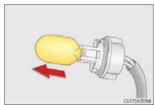
Install a new light bulb then install the bulb base to the light unit by inserting it and turning the bulb base clockwise.
