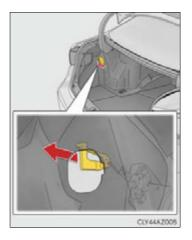
1 After refueling, turn the fuel tank cap until you hear a click. Once the cap is released, it will turn slightly in the opposite direction.
