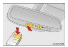
Programming has completed when the indicator light changes to a rapid flash.
