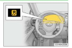
If the vehicle gets stuck in fresh snow or mud, the TRAC system may reduce power from the engine to the wheels. Pressing to turn the system off may make it easier for you to rock the vehicle in order to free it.
