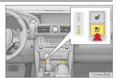
The seat ventilators can be used when the engine switch is in IGNITION ON mode.
