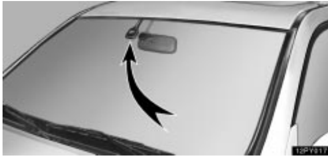
The sensor is on the inside of the windshield as shown above.
