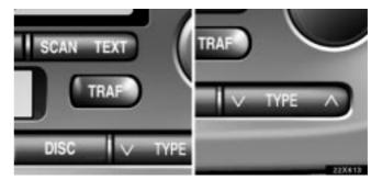
When you push the "TYPE" button, the current program type receiving from RDS station appears on the display.
