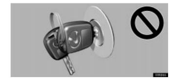
When starting the engine, do not use the key in proximity with other transponder keys (including keys of other vehicles), and do not press other key plates against the key grip. Doing so may prevent the engine from starting, or may cause the engine to stop soon after it starts. If this happens, remove the key once and then insert it again after removing other transponder keys (including keys of other vehicles) from the ring or while gripping or covering them with your hand to start the engine.
