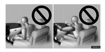
Do not sit on the edge of the seat or lean against the dashboard when the vehicle is in use, since the front passenger airbag could inflate with considerable speed and force. Anyone who is up against, or very close to, an airbag when it inflates, can be killed or seriously injured. Sit up straight and well back in the seat, and always use your seat belt properly.
