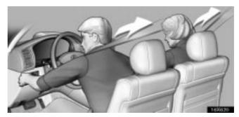
The driver and front passenger seat belt pretensioners are designed to be activated in response to a severe frontal impact or a vehicle rollover.
