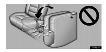
Make sure to stow the third center seat belt in order not to cause damage on the seat belt by pinching it between the third seat inner leg and seat striker.
