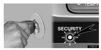
The engine immobilizer system is a theft prevention system. When you insert the key in the ignition switch, the transponder chip in the key's head transmits an electronic code to the vehicle. The engine will start only when the electronic code in the chip corresponds to the registered ID code for the vehicle.
