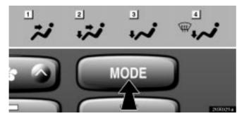
The outlets from which air is delivered can be selected manually by pressing the button. The function of each mode is as follows:
