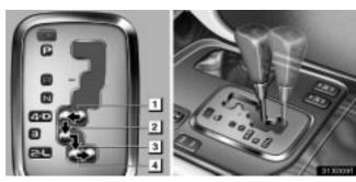
To use the braking power of the engine, downshift the transmission in the way described below:
