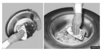
Before putting on the wheel, remove any corrosion on the mounting surfaces with a wire brush or such. Installation of wheels without good metal-to-metal contact at the mounting surface can cause wheel nuts to loosen and eventually cause a wheel to come off while driving. Therefore after the first 1600 km (1000 miles), check to see that the wheel nuts are tight.
