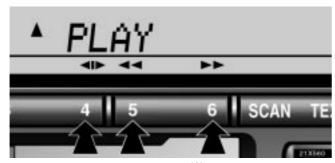
"Program" button: Push the "◀I▶ " button to select the other side of a cassette tape. The display indicates which side is currently selected (▲ indicates top side, ▼ indicates bottom side).
