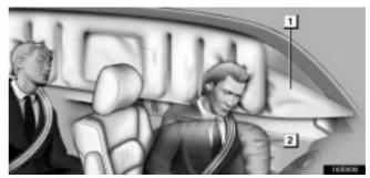
▶ 1 Curtain shield airbag 2 Side airbag
