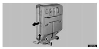
3. Remove the lever cover and pull the lock release lever. Lift up the rear side of the seat and pull the whole seat backward.
