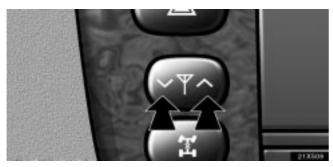
To adjust the height of the antenna manually, push the switch at either side, this may be performed during antenna extension. The maximum extension length is 850 mm (33.5 in.).
