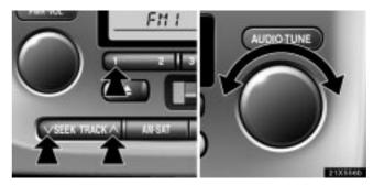
**Preset tuning:** Push the button (1–6) for the station you want. The button number (1–6) and station frequency appear on the display.
