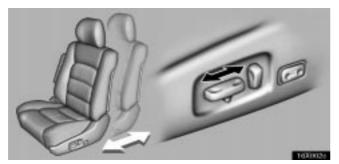
Move the control switch in the desired direction.
