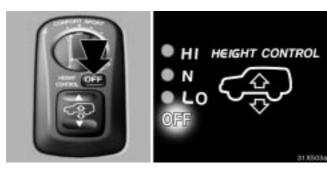
To turn off the active height control suspension with the vehicle stopped, push the height control switch. The height control "OFF" indicator light comes on and the vehicle height is fixed in the same mode as the height control switch is pushed.
