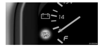
Make sure the roll sensing of curtain shield airbags off indicator is not on. If this indicator light is on, the curtain shield airbags will not inflate in a vehicle rollover and you may be killed or seriously injured.
