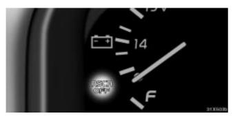
▶ Roll sensing of curtain shield airbags off indicator light
