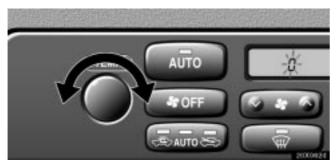
When you turn the "TEMP" knob, the sensitivity changes from "+3" down to "-3". If you do not operate any button for a few seconds or if you push a button other than the air intake control button and temperature control knob, the previous display returns.
