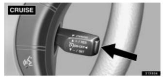
To operate the cruise control, push the main switch. This turns the system on. The indicator light in the instrument cluster shows that you can now set your desired cruising speed. Another push on the switch will turn the system completely off.
