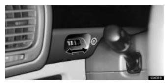
To adjust the brightness of the instrument panel lights, turn the dial.
