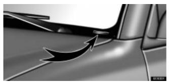
The vehicle identification number (VIN) is the legal identifier for your vehicle. This number is on the left top of the instrument panel and can be seen through the windshield from outside.
