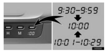
The digital clock indicates the time when the ignition key is at the "ACC" or "ON" position. To reset the hour, press the "H" button. To reset the minutes, press the "M" button. To adjust the time to the nearest hour, press the ":00" button.
