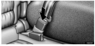
4. To remove the infant seat, press the buckle release button and allow the belt to retract completely. The belt will move freely again and be ready to work for an adult or older child passenger.
