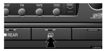
To turn the electric outside rear view mirror defogger on, push the switch.
