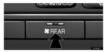
To turn on the rear air conditioning when you sit on the front seat, push this switch. The rear air conditioning operates in the automatic mode. To adjust the air flow and setting temperature, follow the steps in accordance with "Rear air conditioning controls" on page 205.
