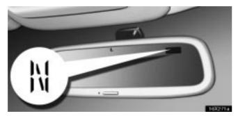
The compass indicates the direction in which the vehicle is heading. The illustration shown above indicates that the vehicle is heading north.
