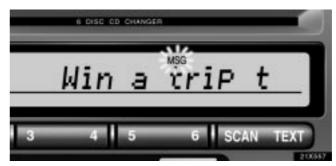
If the radio receives a radio text from RDS station, "MSG" appears on the display. Push the "TEXT" button, and a text message is displayed.
