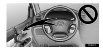
Do not attach a cupholder or any other device or object on or around the door. When the side airbag inflates, the cupholder or any other device or object will be thrown with great force, or the side airbag may not activate correctly, resulting in death or serious injury. Likewise, the driver and front passenger should not hold objects in their arms or on their knees.
