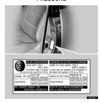
The recommended cold tire inflation pressures, tire size and the combined weight of occupants and cargo (vehicle capacity weight) are described on the tire and loading information label.
