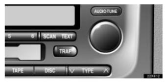
Each time you push the "AUDIO-TUNE" knob, the display changes as in the following. To adjust the tone and balance or turn on or off the automatic sound levelizer, turn the knob.
