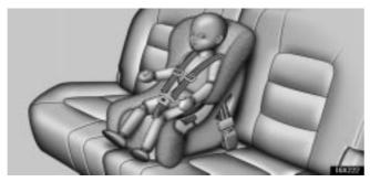
A convertible seat must be used in forward–facing and rear–facing positions depending on the age and size of the child. When installing, follow the manufacturer's instructions about the appropriate age and size of the child as well as directions for installing a child restraint system.
