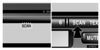
To scan the currently selected channel category: Push the "SCAN" button briefly. "SCAN" appears on the display. The radio will find the next channel in the same channel category up the band, stay there for a few seconds, and then scan again. To select a channel, push the "SCAN" button a second time.
