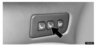
When you push button "1" or "2", the driving position will be automatically adjusted to the position recorded for that button.
