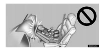
Never install a rear-facing child restraint system on the front passenger seat. In the event of an accident, the force of the rapid inflation of the front passenger airbag can cause death or serious injury to the child if the rear-facing child restraint system is installed on the front passenger seat.
