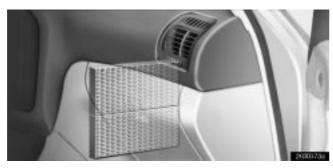
Your vehicle is equipped with an air conditioning filter. The air conditioning filter may clog after long use and reduce the air flow quantity.
