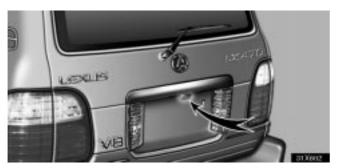
The rear view monitor system camera is located on the back door as shown in the illustration. The camera uses a special lens. The distance of the image that appears on the screen differs from the actual distance.
