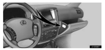
The air conditioning filter information label is placed on the left side of the glove box as shown and indicates that a filter has been installed.
