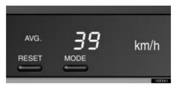
The following information is shown with the ignition switch turned on. Each time you push the "MODE" button, the displayed information is changed.
