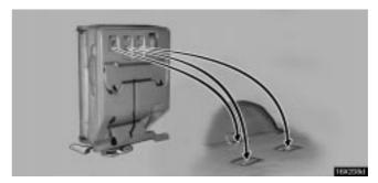
4. Remove the seat hook covers from the back of the seat cushion and install them onto the seat anchor brackets.
