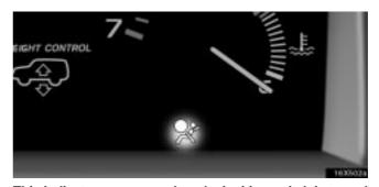
This indicator comes on when the ignition switch is turned to the "ON" position. It goes off after about 6 seconds. This means the seat belt pretensioners are operating properly.
