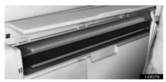
This auxiliary box is equipped with a band to hold the warning reflector.
