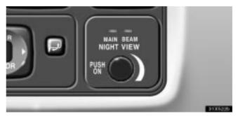
The Lexus night view system turns on and the "MAIN" indicator light comes on when you push the knob with the ignition switch on:
