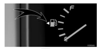
The arrow head next to as shown indicates on which side of your vehicle the fuel filler door is located.
