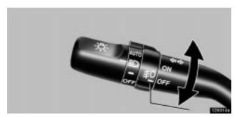
To turn on the fog lights, turn the switch to the "ON" position. They will come on only when the headlights are on low beam.
