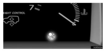
This indicator comes on when the ignition switch is turned to the "ON" position. It goes off after about 6 seconds. This means the SRS side airbags and curtain shield airbags are operating properly.
