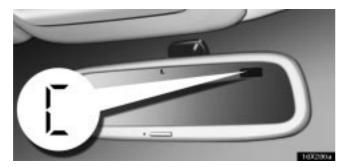
"C" appears on the display in case the circling calibration is required due to a drastic change in the magnetic field. To rectify this, follow the calibration procedure below.
