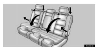
1. Lower the head restraints to the lowest position, unlock the seatback by pulling the lever on the side of the seatback and fold it down.
