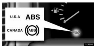
The light comes on when the ignition key is turned to the "ON" position. If the anti-lock brake system and the brake assist system work properly, the light turns off after a few seconds. Thereafter, if either of the systems malfunctions, the light comes on again.
