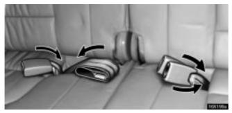
Before removing the third seats, stow the third seat belt and buckles as shown in the illustration.
