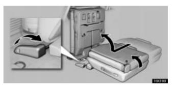
2. While turning the lever, lift and slide the whole seat backward.
