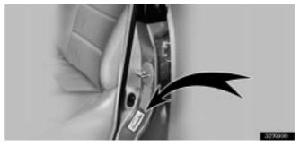
The vehicle identification number (VIN) is also on the Certification Label.
