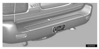
A tow hitch receiver should be installed as shown before towing.
