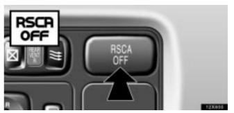
► Roll sensing of curtain shield airbags off switch
