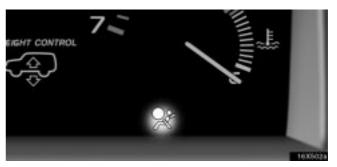
This indicator comes on when the ignition switch is turned to the "ON" position. It goes off after about 6 seconds. This means the SRS front airbags are operating properly.
