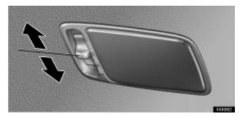
To turn on the interior light, slide the switch.
