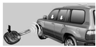
Push the "UNLOCK" button until the windows and moon roof start to move. At this time one beep sounds. When you release the button, the windows and moon roof stop operating.
