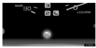
The vehicle stability control system helps provide integrated control of the systems such as anti-lock brakes, traction control, engine control, etc. This system automatically controls the output of the brakes or engine to help prevent the vehicle from skidding under adverse conditions.
