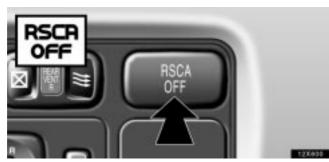
The roll sensing of curtain shield airbags off switch can turn off the curtain shield airbags and front seat belt pretensioners in a vehicle rollover. This switch should only be used in a situation where the inflation is not desired (such as during extreme offroad driving).
