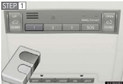
Point the remote control transmitter for the device 1 to 3 in. (25 to 75 mm) from the HomeLink® buttons.
