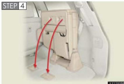
Remove the seat hook covers from the underside of the seat cushion, and install them on the seat hooks.
