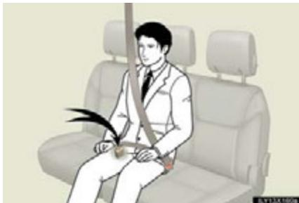
Make sure that the buckle with the gray buckle release button is securely latched for ready use of the center seat belt.
