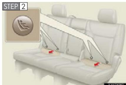
Take off the covers between the seat cushion and seatback, then confirm the position of the LATCH anchors below the symbol in the seatback.
