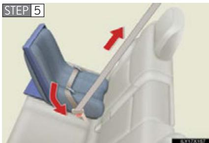
While pushing the child restraint system down into the second seat, allow the shoulder belt to retract until the child restraint system is securely in place.
