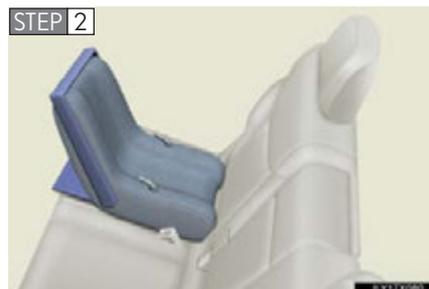
Place the child restraint system on the second seat facing the rear of the vehicle.
