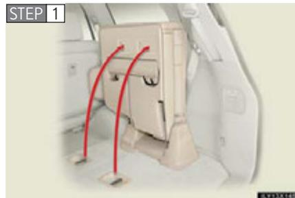
Remove the seat hook covers from the floor and install them into the underside of the seat cushion.
