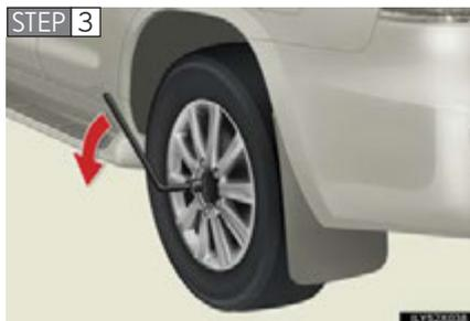
Slightly loosen the wheel nuts (one turn).
