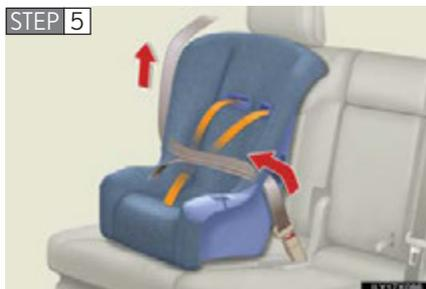
While pushing the child restraint system into the second seat, allow the shoulder belt to retract until the child restraint system is securely in place.
