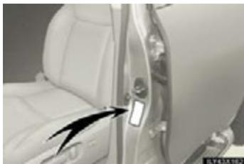
For the GAWR, see the Certification Label. For the maximum load of the tire, see the load limit at maximum cold tire inflation pressure mentioned on the sidewall of the tire. (→P. 707)
