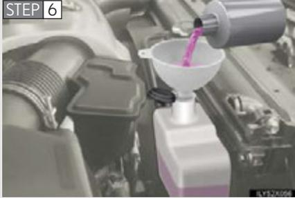
Add engine coolant if necessary.
