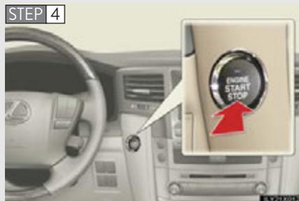
Press the “ENGINE START STOP” switch.
