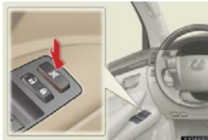
Press the switch down to lock passenger window switches.
