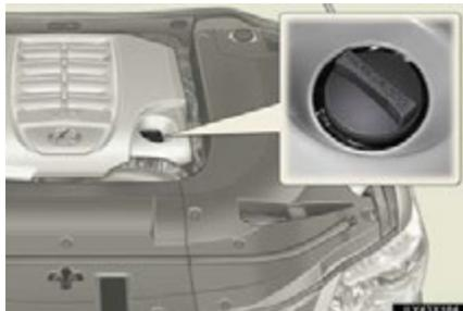
If the oil level is below or near the low level mark, add engine oil of the same type as already in the engine. (→P. 697)
