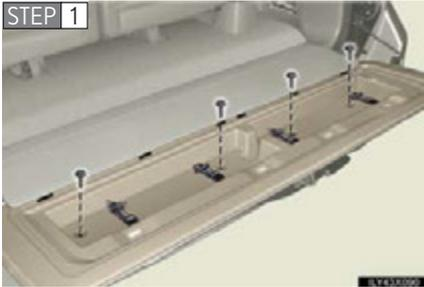
Open the back door and remove the bolts and the cover.
