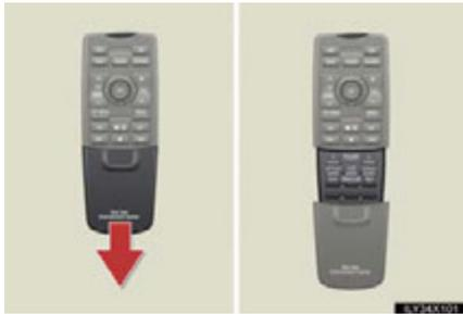
To use the buttons under the cover, slide the cover down.
