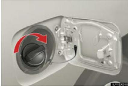
When replacing the fuel tank cap, turn it until a clicking sound is heard.
