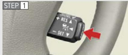
Press the "ON-OFF" button to activate the cruise control.
