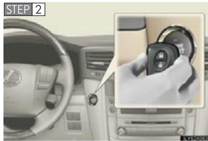
**STEP 2** Touch the Lexus emblem side of the electronic key (including the card key) to the “ENGINE START STOP” switch.
