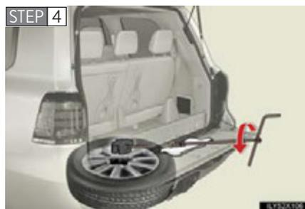
Lower the spare tire completely to the ground.
