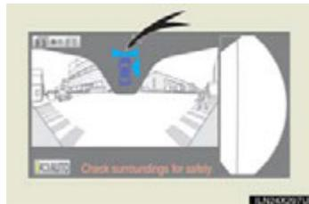
If the wide view front & side monitor is switched to from the Lexus parking assist monitor, the icon display area will flash to inform the driver that the currently displayed area is the front or side. The icon display area will continue to flash until the screen is turned off.
