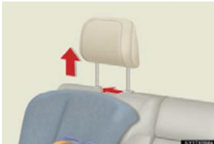
Adjust the head restraint to the upmost position.
