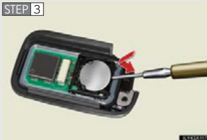
Remove the depleted battery.
