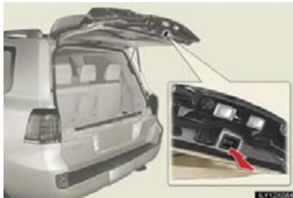
Pressing the switch closes upper back door automatically. (A buzzer sounds)
