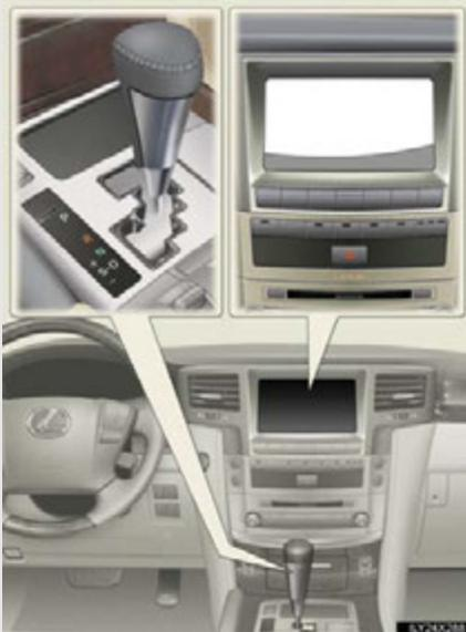
Rear view image is displayed when the shift lever is in "R".
