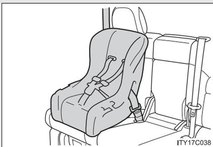
Seat belts equipped with a child restraint locking mechanism (ALR/ELR belts except driver's seat belt) (→P. 72)
