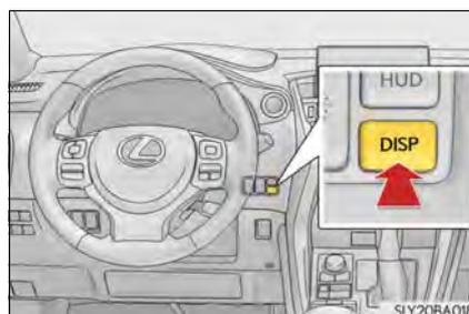
On and off will be switched between each time the button is pressed.
