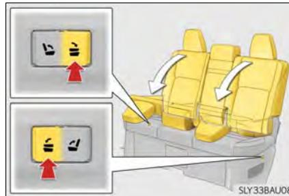
When the seatback is collapsed to the rear, put the seatback in the most upright position and press the switch once again.
