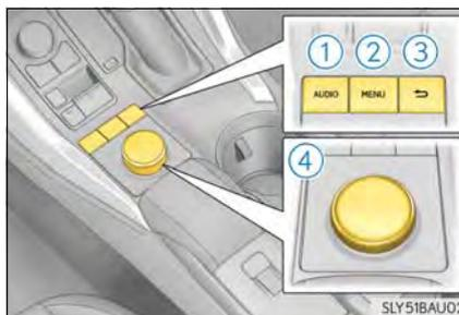
Move the controller to display the left or right side of the screen.
