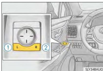
**2** To adjust the mirror, press the switch.
