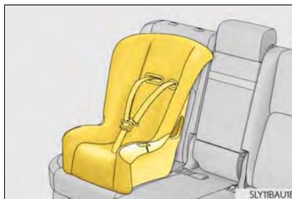
**4** Run the seat belt through the child restraint system and insert the plate into the buckle. Make sure that the belt is not twisted.
