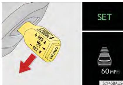
While the vehicle is in vehicle-to-vehicle distance control mode, if the lever is released when vehicle speed is less than 30 mph (50 km/h) and a vehicle ahead can be detected, the vehicle will start following the vehicle ahead at a set speed of 30 mph (50 km/h).
