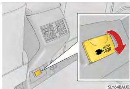
The power outlet can be used when the power switch is in ON mode.
