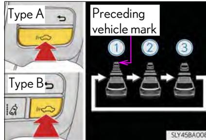
**Vehicle-to-vehicle distance settings (vehicle-to-vehicle distance control mode)**
