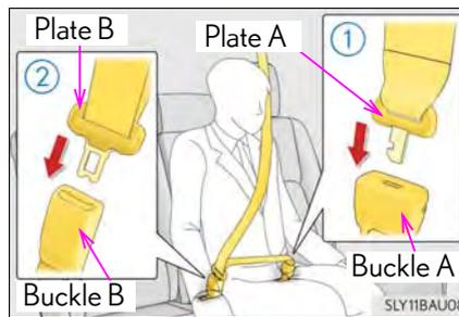
**Releasing and stowing the seat belt (for the rear center seat)**
