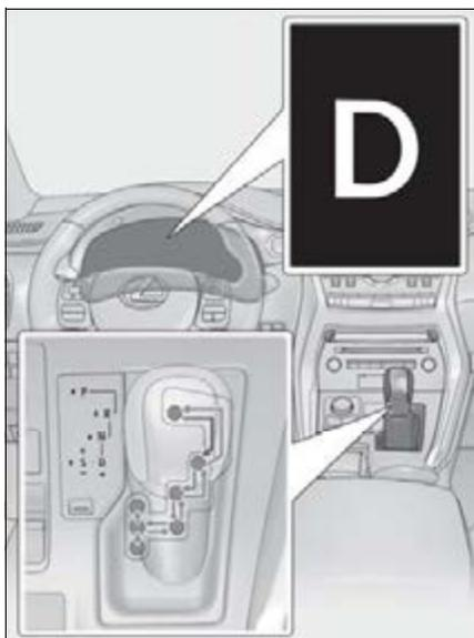
← While the power switch is in ON mode, move the shift lever with the brake pedal depressed. When shifting the shift lever between P and D, make sure that the vehicle is completely stopped.
