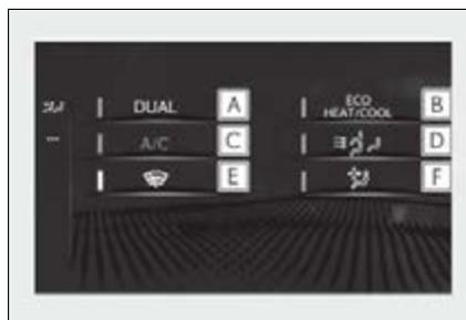
**A** Adjusting the temperature for driver and passenger seats separately (“DUAL” mode) (→P.272)
