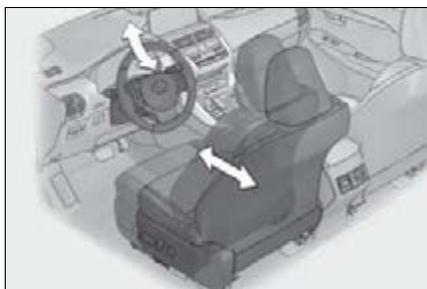
When all of the following have been performed, the driver's seat and steering wheel are automatically adjusted to a position that allows driver to enter and exit the vehicle easily.
