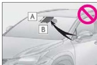
**A** From the top of the windshield to approximately 0.4 in. (1 cm) below the bottom of the camera sensor
