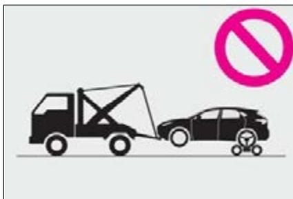
**Towing with a wheel-lift type truck**
