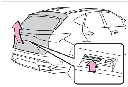
Lift the back door while pressing the back door opener switch.
