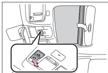
\*1: Lightly press either end of the moon roof
