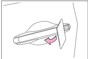
**2 Remove the cover by pressing it on the rear.**
