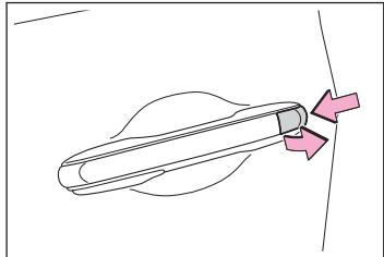
**3 Using the mechanical key, turn the lock cylinder to the unlock side to enable the manual release handle operation.**
