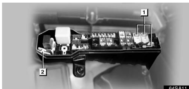
□ Engine compartment 1 Spare fuses 2 Pull-out tool
