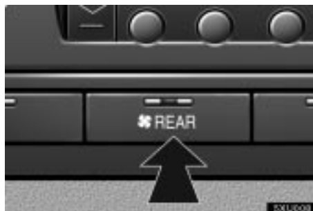
(c) Rear air conditioning switch
