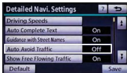
**step 3** Select **On** from the Auto Avoid Traffic option. Touch **Save** followed by **↶**. The system will automatically select another route when moderate or heavy traffic is detected during route guidance.
