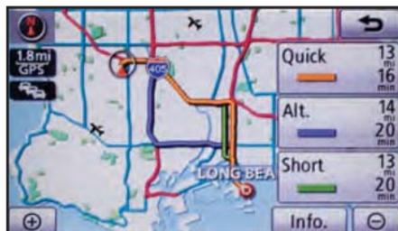
One of three routes may be chosen for the trip. Quick offers the shortest route by time; Alt. is the second fastest route; Short is the most direct based upon driven mileage. The system does not account for traffic signals or traffic flow.
