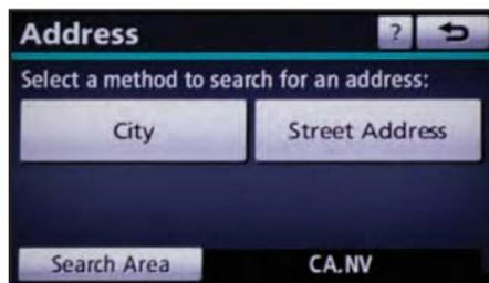
Prior to inputting the desired address select the Search Area by pressing **Search Area**. If the incorrect Search Area is chosen, the system will either find an address that closely matches in that area or will indicate that the address cannot be found.
