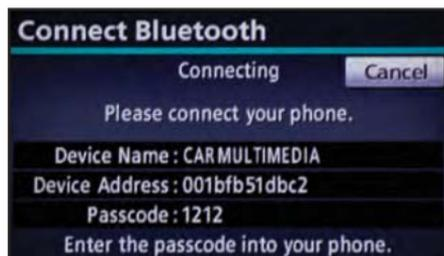
**step 3** Input the passkey listed on the screen into the approved Bluetooth cell phone. Please refer to the cell phone manufacturer's user guide for pairing procedures.
