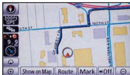
Touch **Show on Map** to select from seven different screen viewing options. Four screen preferences are available when the map is visible and three additional are available during route guidance only.
