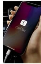
**STEP 2** Plug a compatible iPhone® into the USB media port using an Apple® approved cable.
