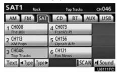
To scan the currently selected channel category: Touch "SCAN" briefly. "SCAN" appears on the display. The radio will find the next channel in the same channel category, stay there for a few seconds, and then scan again. To select a channel, touch "SCAN" a second time.
