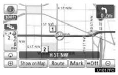
The current vehicle position mark  $(\boxed{1})$  appears in the center or bottom center of the map screen.
