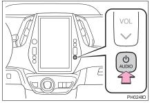
**"AUDIO"** button: Press to turn the audio system on and off. The system turns on in the last mode used.
