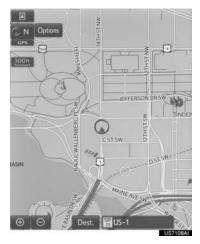
When the vehicle is receiving signals from satellites, the "GPS" mark appears at the top left of the screen.
