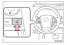
The voice command system and its list of commands can be operated. (→P.132)
