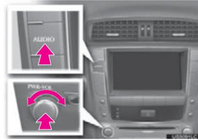
“AUDIO” button: Press to display screen buttons for the audio/video system.
