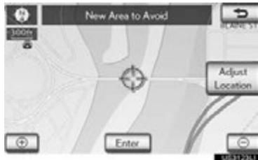
**“Adjust Location”:** Touch to adjust the position in smaller increments.
