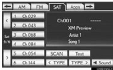
**To scan the currently selected channel category:** Touch “SCAN”. “SCAN” appears on the screen. The radio will find the next channel in the same channel category, stay there for a few seconds, and then scan again. To select a channel, touch “SCAN” again.
