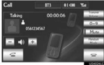
**To adjust the volume of the other party's voice:** Touch “-” or “+”, turn the “PWR·VOL” knob, or use the volume switch on the steering wheel.
