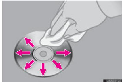
**To clean a disc:** Wipe it with a soft, lint-free cloth that has been dampened with water. Wipe in a straight line from the center to the edge (not in circles). Dry it with another soft, lint-free cloth. Do not use a conventional record cleaner or anti-static device.
