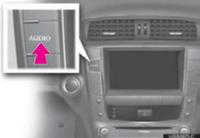
2 Touch the "DISC" tab or press the "AUDIO" button repeatedly until the "DISC" tab is selected.
