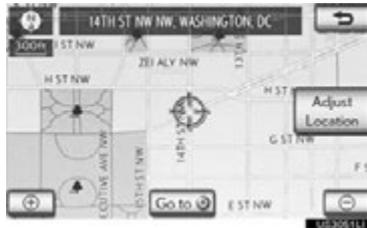
**“Adjust Location”**: Touch to adjust the position in smaller increments.
