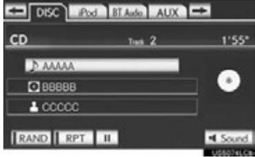
"PRST-TRACK" button: Press the ">" or "<" button of "PRST-TRACK" repeatedly until the desired track number appears on the screen. The player will start playing the selected track from the beginning.
