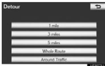
**"1 mile (km)", "3 miles (km)" or "5 miles (km)":** Touch one of these screen buttons to start the detour process. After detouring, the system returns to the original guidance route.
