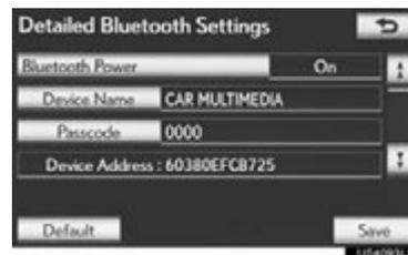
2 Use the software keyboard to input the device name and touch “OK”.
