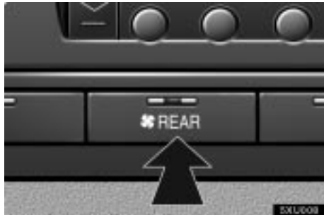
(c) Rear air conditioning switch
