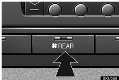
(c) Rear air conditioning switch
