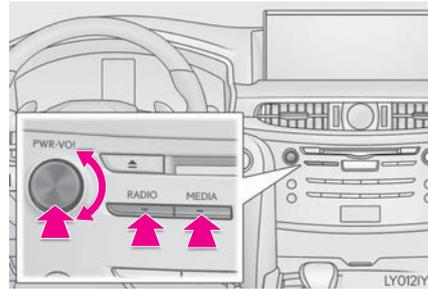
**“PWR·VOL” knob:** Press to turn the audio/visual system on and off. The system turns on in the last mode used. Turn this knob to adjust the volume.
