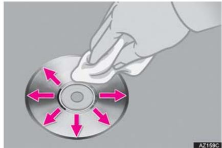
**To clean a disc:** Wipe it with a soft, lint-free cloth that has been dampened with water. Wipe in a straight line from the center to the edge of the disc (not in circles). Dry it with another soft, lint-free cloth. Do not use a conventional record cleaner or anti-static device.
