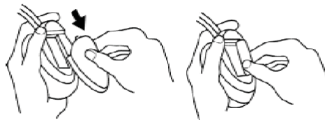
Figure 3. Replacing the Headphone Batteries
